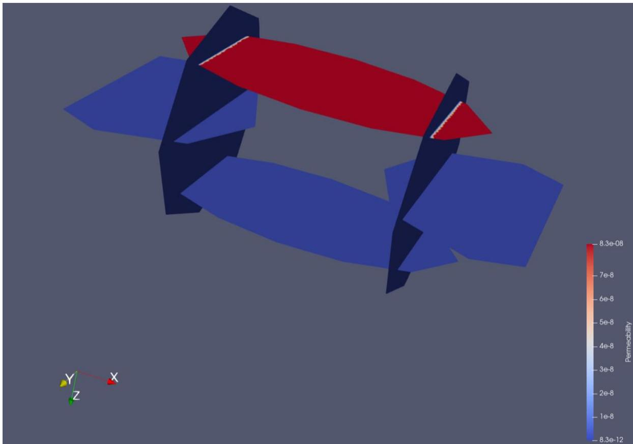
**Figure 1. Initial model for discrete fracture networks (permeability)**
