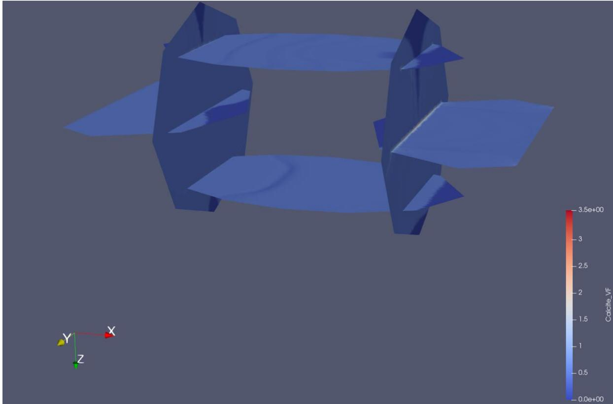
**Figure 8. Chemistry model for discrete fracture networks (calcite volume fraction at time = 50 days)**
