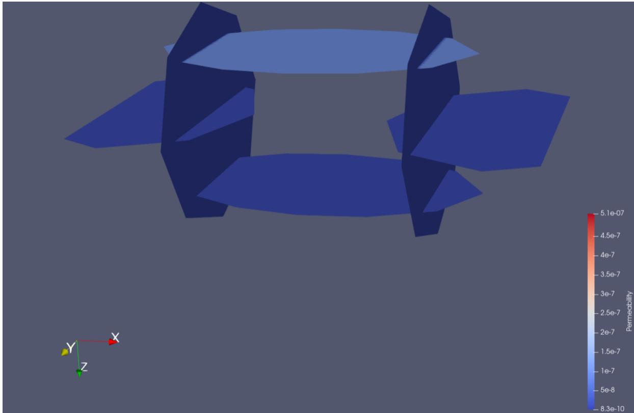
**Figure 2. Chemistry model for discrete fracture networks (permeability at time = 0 days)**
