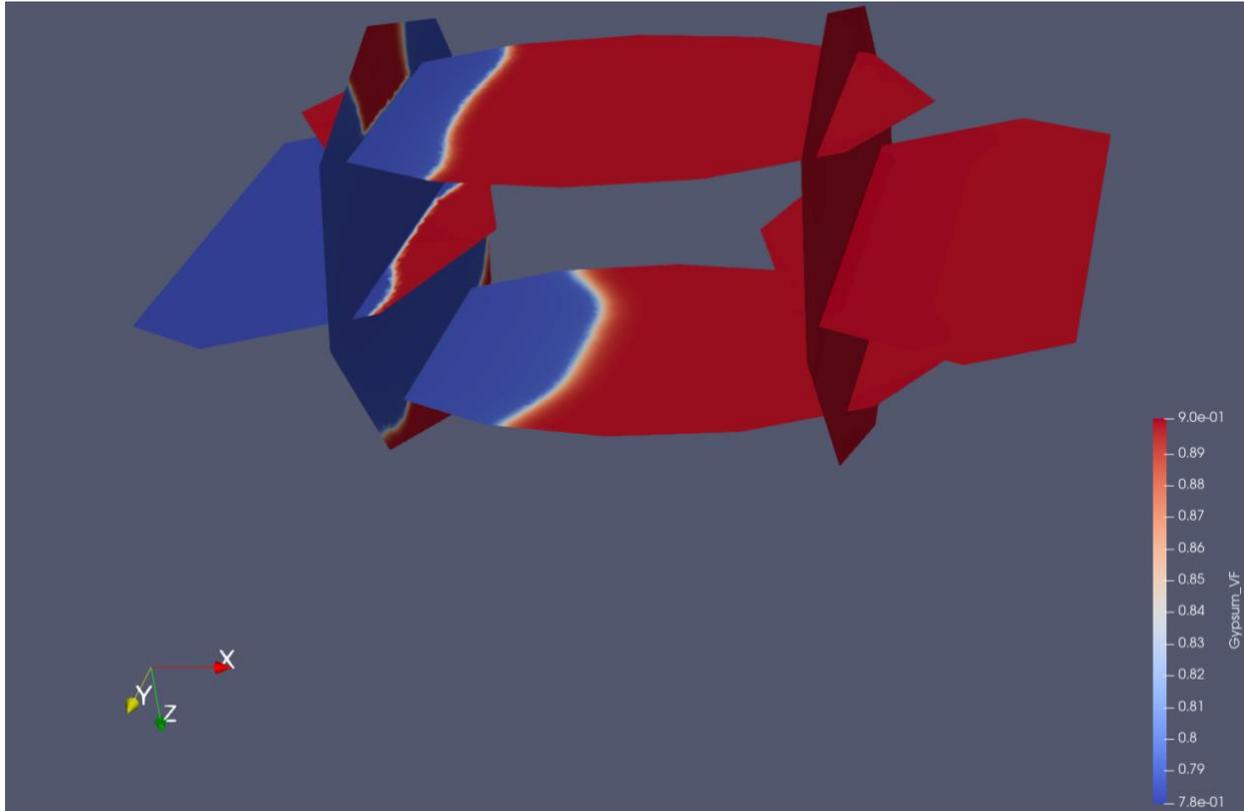
**Figure 5. Chemistry model for discrete fracture networks (gypsum volume fraction at time = 1 day)**
