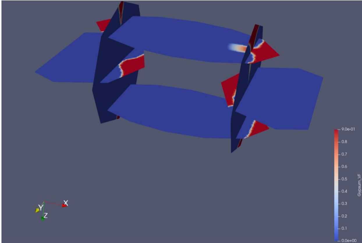
**Figure 7. Chemistry model for discrete fracture networks (gypsum volume fraction at time = 50 days)**
