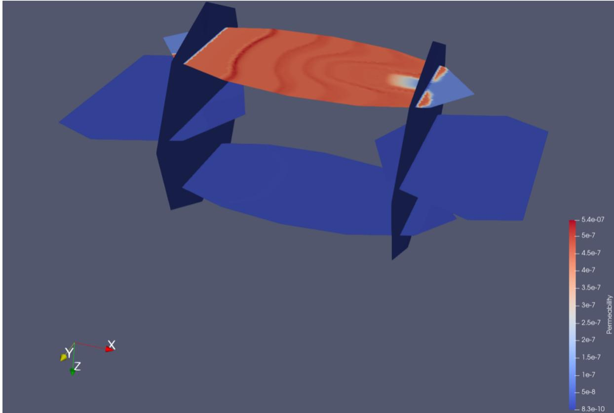
**Figure 9. Chemistry model for discrete fracture networks (permeability at time = 50 days)**
