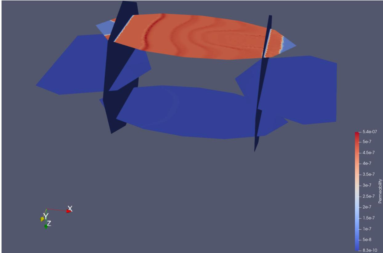
**Figure 10. Chemistry model for discrete fracture networks (permeability at time = 100 days)**
