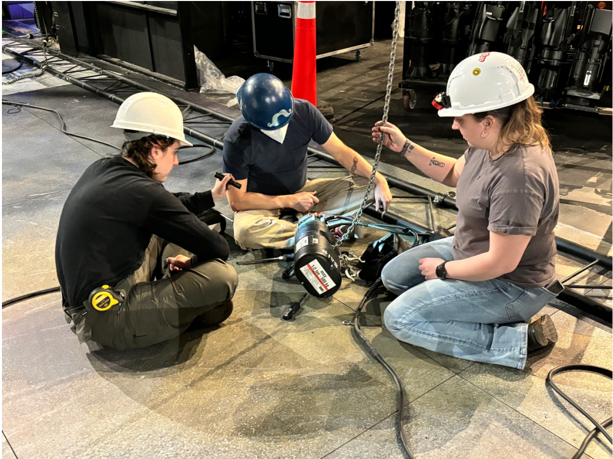
Figure 42: Chris, Ashley, and I working on fixing the chain motors
