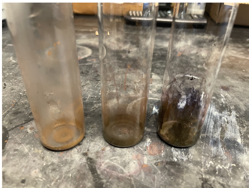
Figure A.8: AuNP decomposition was observed visually. The as-synthesized AuNP product appears black (right).
