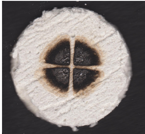
Figure 2.2: Alumina target used for laser alignment.
