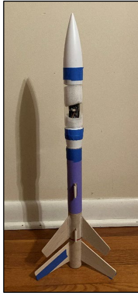
Figure 4.9. Low-Power Rocket with Sensors in Electronics Bay
