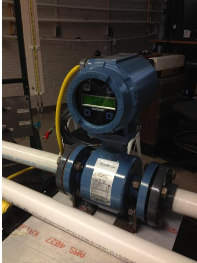
Figure 15 - A picture of the flow meter during the head loss test of the commercial valve
