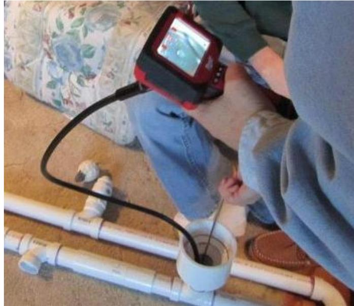
**Figure 13 - Picture of the valve seating monitor via the Milwaukee fiber-optic camera**
