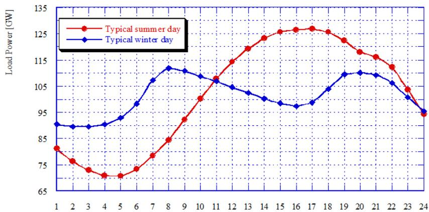
Figure 5: Load profile for PJM service area, for a typical summer and winter day [9]
