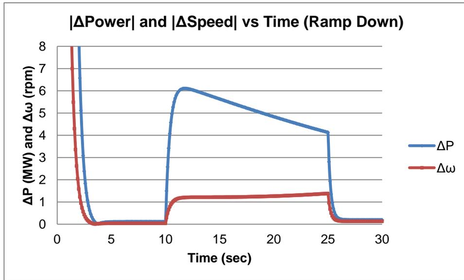
Figure 16:  $\Delta$ Power and  $\Delta$ Speed vs Time (Ramp Down)
