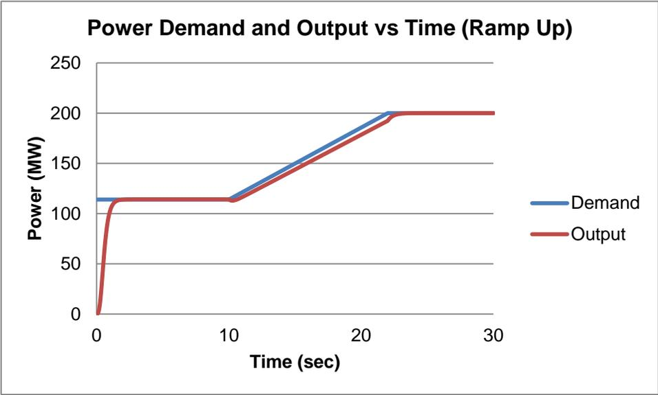
Figure 13: Power Demand and Output vs Time (Ramp Up)
