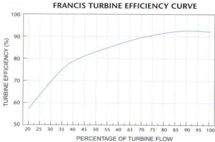
Figure 7: Francis Turbine Efficiency Curve [14]
