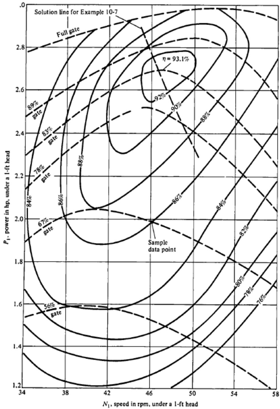
Figure 26: Efficiency hill for a Francis Turbine [13]
