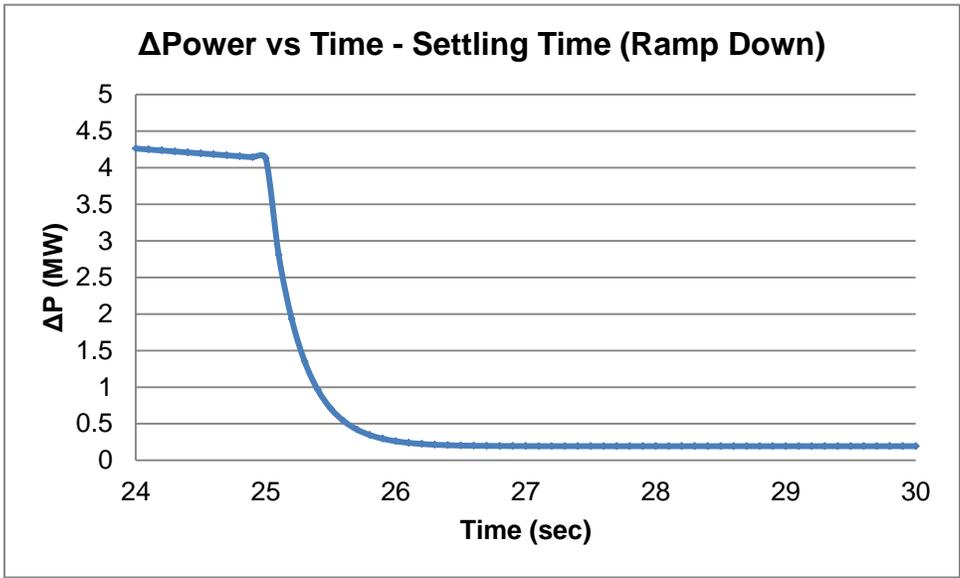
Figure 18: ΔPower vs Time - Settling Time (Ramp Down)
