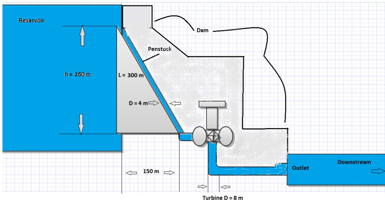
Figure 12: Sketch of the Model Plant
