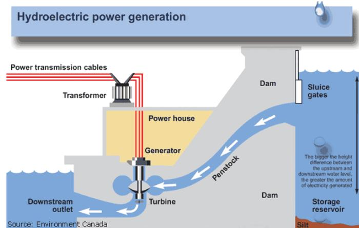
Figure 3: Schematic of a Simplified Hydroelectric Power Plant [6]
