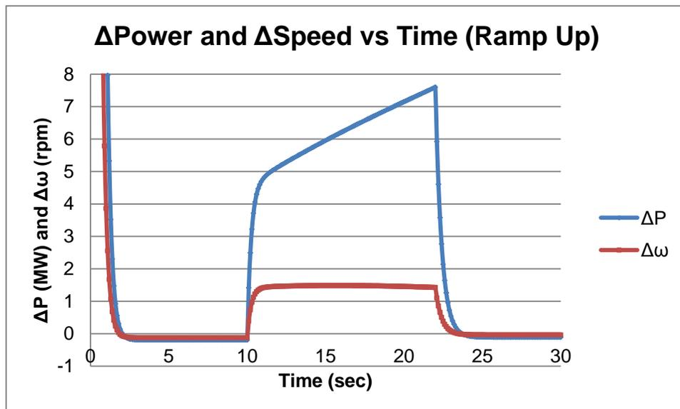
Figure 15: ΔPower and ΔSpeed vs Time (Ramp Up)
