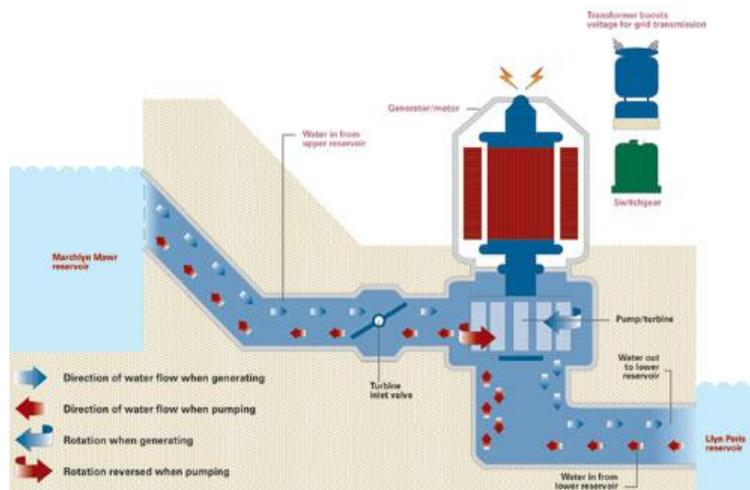
Figure 4: Water Flow for Generation and Pumping [7]
