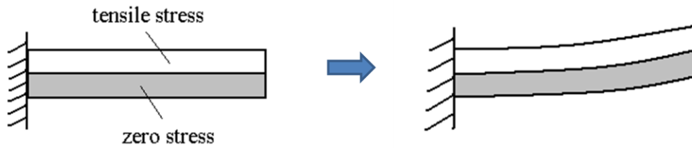
Figure 2.1.3 (a) Cantilever bending upward due to tensile residual stress
