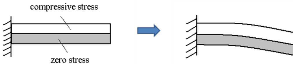
Figure 2.1.3 (b) Cantilever bending downward due to compressive residual stress
