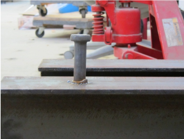
Figure 1-2 Headed Shear Stud
