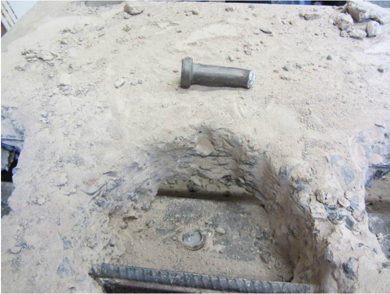
Figure 5-6 Shear Stud after Low Impact with Sledge Hammer
