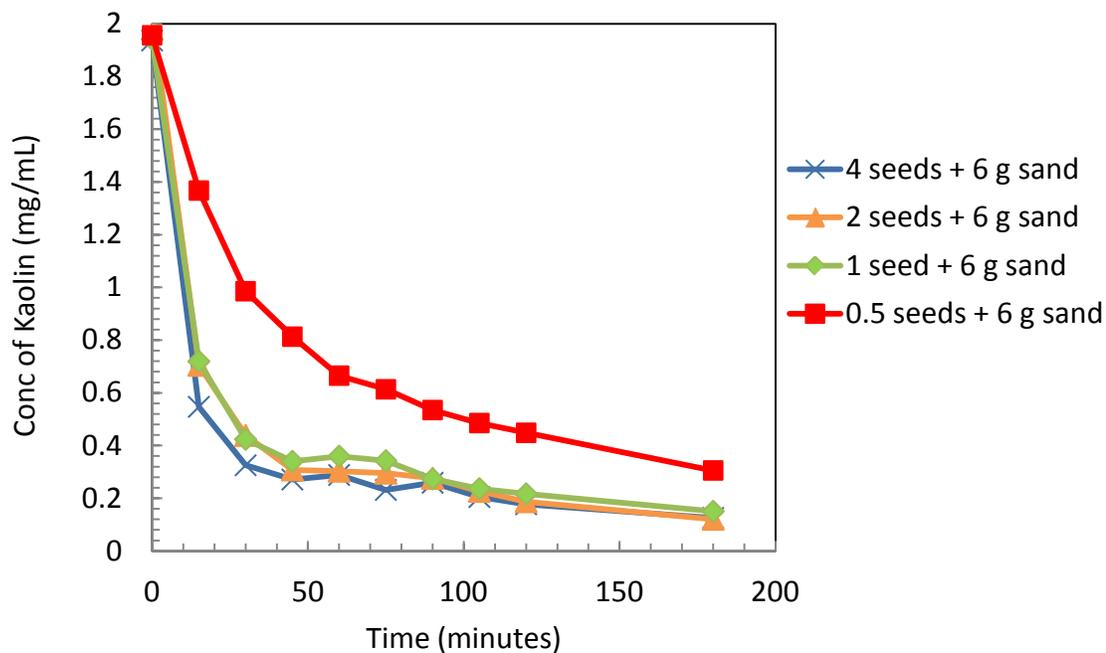
**Figure 4.** Preparation of *f*-sand was optimized to reduce Moringa seed usage by 75%. 1 seed can be used to functionalize 6 grams of sand and achieve the same kaolin clearance as the initial formulation (4 seeds to functionalize 6 grams of sand).
