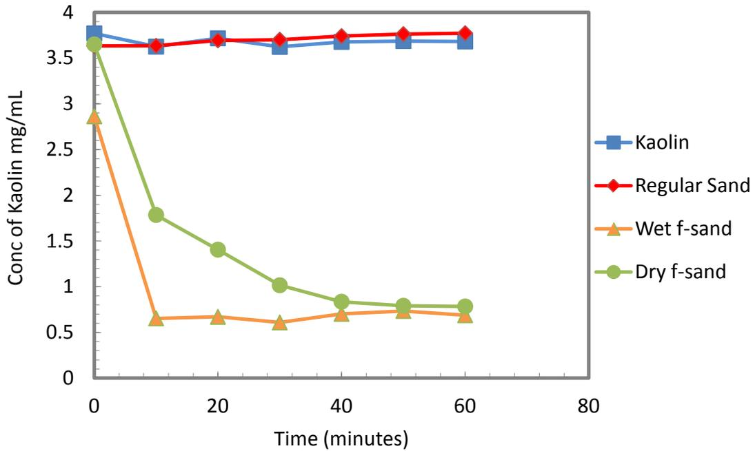
**Figure 5.** Kaolin removal ability of wet and dry stored sand is compared. Wet and dry stored sand both achieve significant kaolin removal compared to plain sand and untreated kaolin solution. The dry stored sand follows a shallower curve and does not achieve as much kaolin removal in the first 40 minutes. This graph shows average removal of at least 10 samples prepared in triplicate for both the wet and dry sand.
