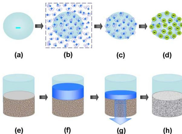
**Figure 2.** Process for production of *f*-sand. The process is shown on the individual sand grain (a-d) and for the batch process (e-h). The anionic sand grains (a, e) are soaked with Moringa serum containing MOCP (b, f). After removal of the Moringa serum, the MOCP remains adhered to the surface of the sand grains (c, g). Anionic particles, including bacteria, can then adhere to the cationic functionalized sites on the sand grains (d, h)<sup>i</sup>.
