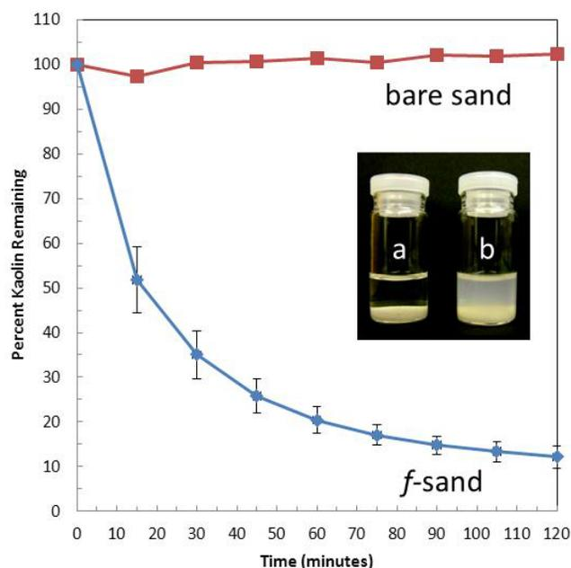
**Figure 3.** Kaolin is removed from solution using *f*-sand and no removal is measured when kaolin solution is treated with bare sand. The average removal rate was 83% of kaolin in one hour using 2 grams of *f*-sand. Inset: the kaolin removal of *f*-sand is demonstrated. (a) *f*-sand treated kaolin suspension. (b) the same suspension treated with bare sand. The *f*-sand treated sample is visibly less turbid than the sample treated with bare sand<sup>1</sup>.
