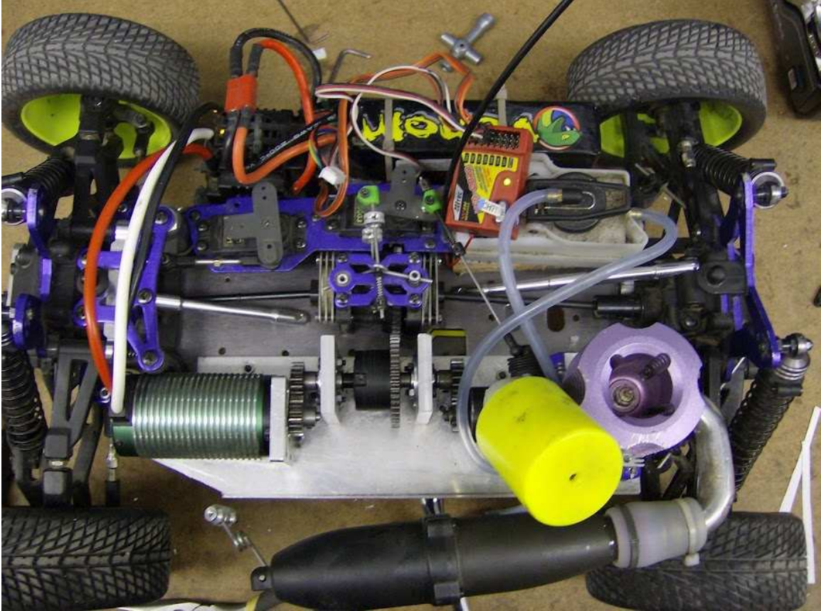
Figure 6: Hybrid nitro/electric RC car constructed at the University of Kansas [6].
