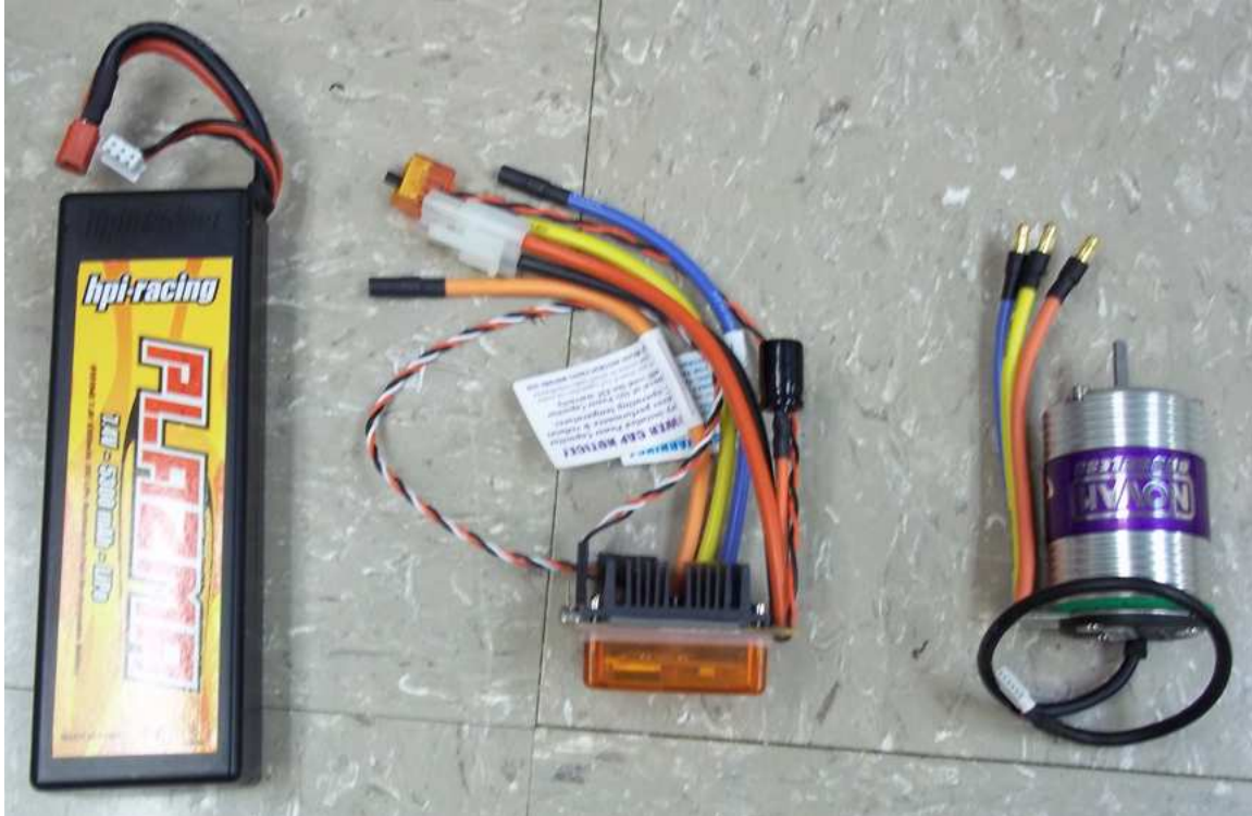
Figure 8: Components of the electric drivetrain, from left to right: battery, ESC, motor.
