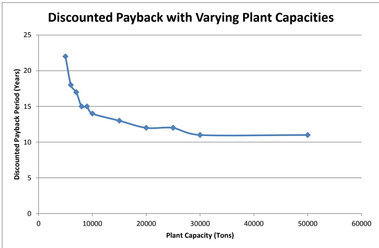
Figure 8: Calculated discounted payback period for varying plant capacities in Model 2 (Piping length remained constant, effectively varying load density)
