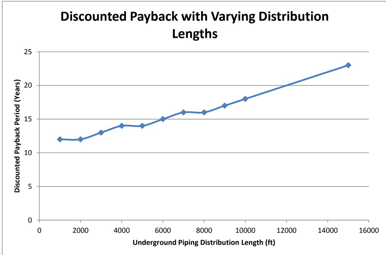
**Figure 9: Calculated discounted payback period for varying pipe distribution lengths (Plant capacity remained constant, effectively varying load density)**
