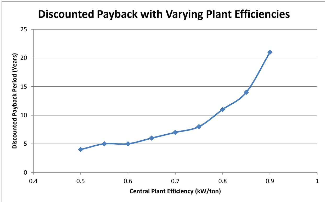
**Figure 10: Calculated discounted payback period for varying district energy central plant efficiencies**
