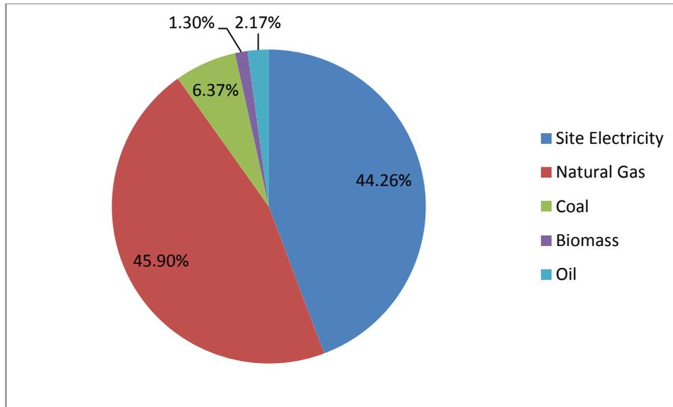
Figure 4: U.S. district cooling fuel consumption by fuel type, 2003 (US EIA, 1999)
