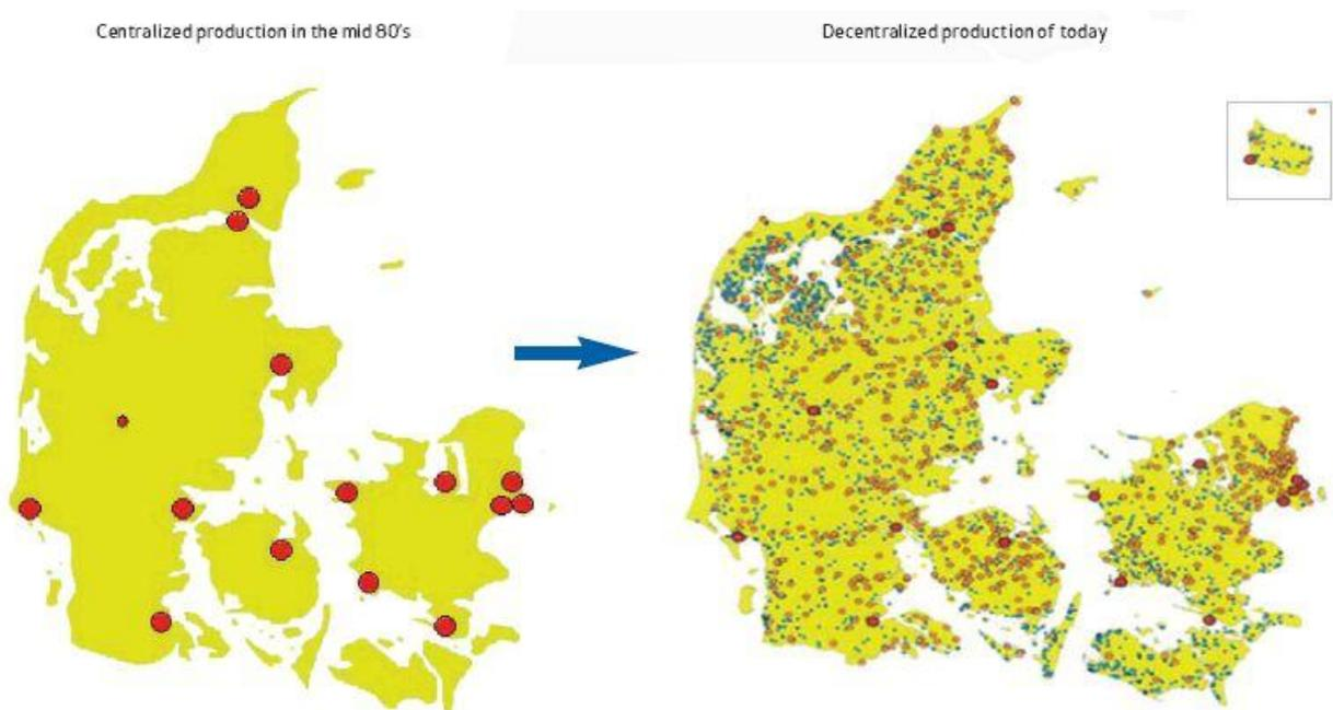
**Figure 7: Decentralization of Denmark's electricity generation in the past few decades (The International CHP/DHC Collaborative: Denmark Scorecard, 2007)**
