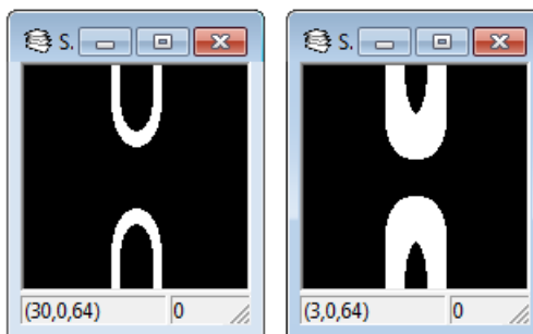
Fig. 3.4. A sample slice of Curve_Branch_Tube before (left) and after (right) binary morphological dilation using the binaryMorph_Dilate function.
