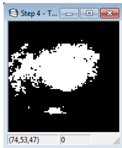
Fig. 5.6. A slice of image r1a after connected component labelling with an increased minimum region size. This is the result of the script in Figure 5.5.
