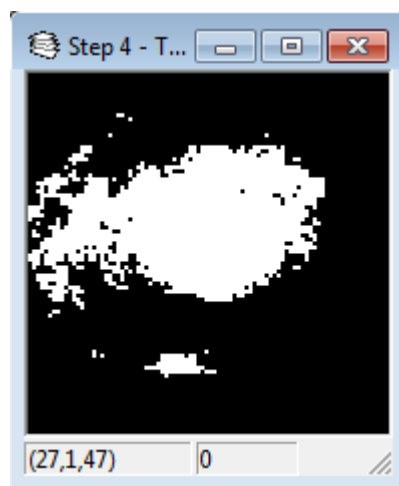
Fig. 5.4. A slice of image r1a after connected component labelling. This is the result of the script in Figure 5.3.
