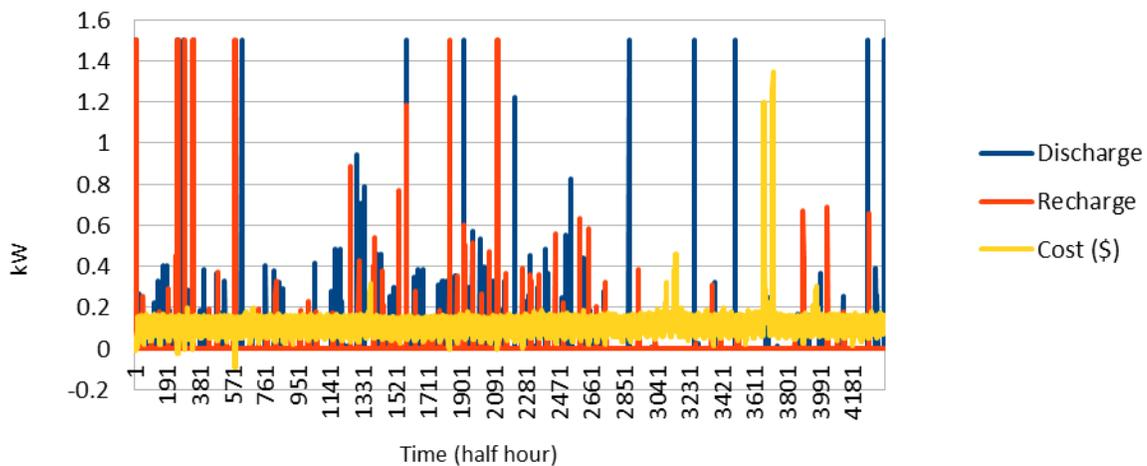
Figure A.3 – Graph of battery recharge and discharge.
