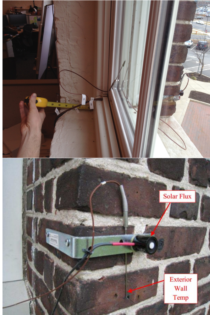
Figure 1.2. Installation apparatus for the LI200X pyranometer on the East Wall of B101.
