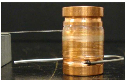
**Figure 3: Glass fiber wound on a copper spool**
