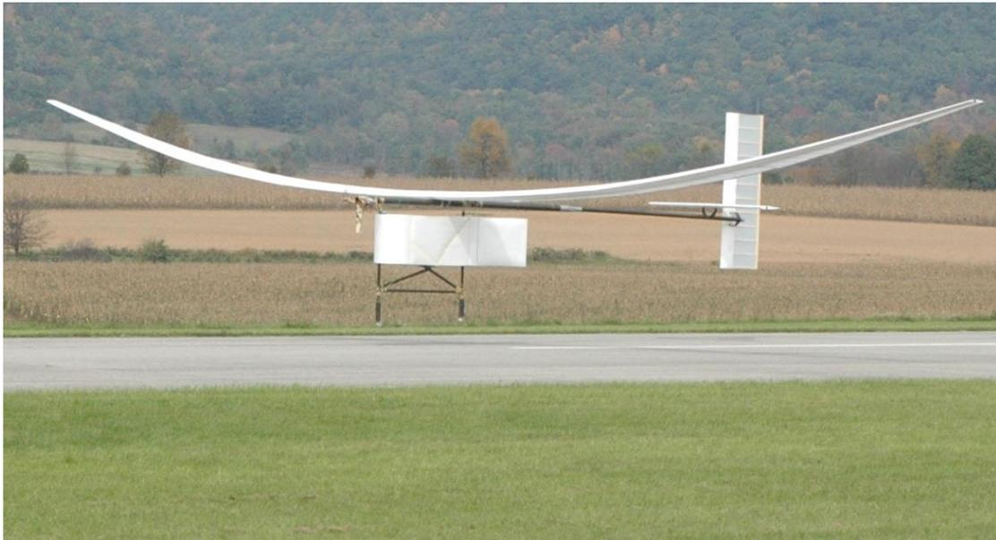
**Figure 2-1.** *Zephyrus* Flight Test Photo. Flown with 140 lb ballast and under radio control. This flight test took place in the spring of 2012.
