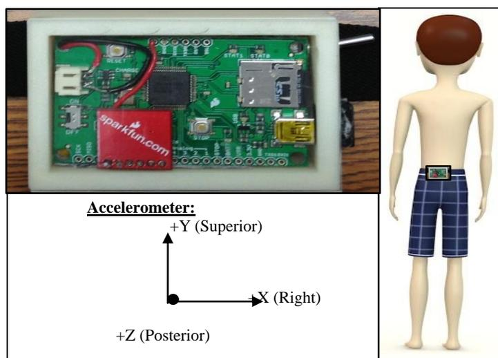
Figure 5-6: Beta Prototype Orientation
