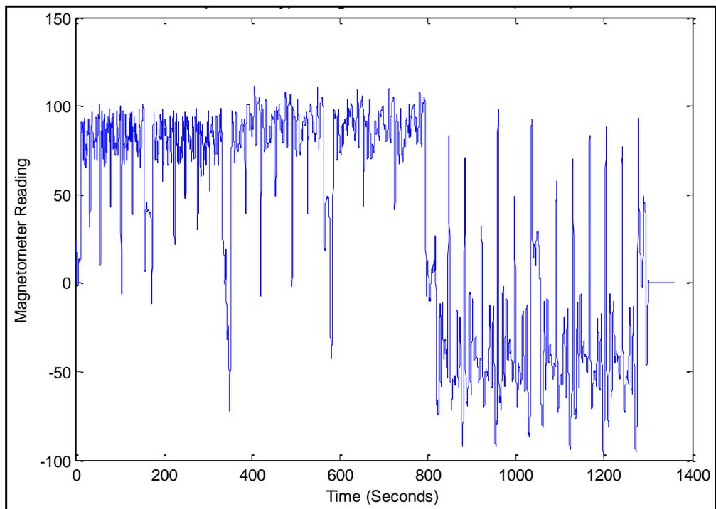
Figure B-9: Alpha Prototype Magnetometer Axis 3 Data (2<sup>nd</sup> Order Butterworth Filter Applied)
