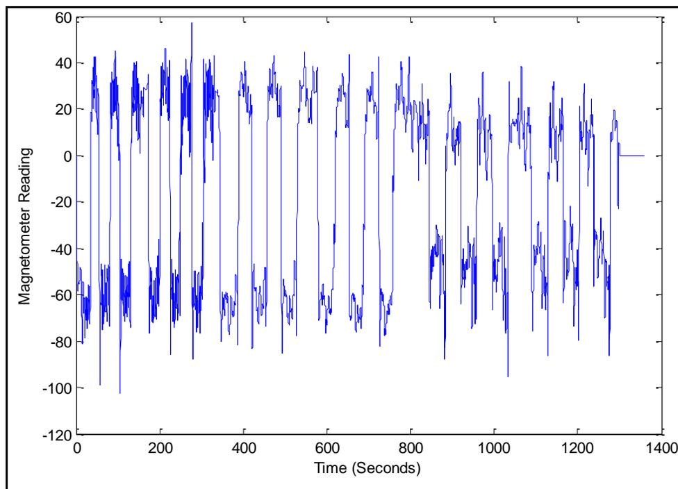
**Figure 5-2: Alpha Prototype Magnetometer Axis 1 Data (2<sup>nd</sup> Order Butterworth Filter Applied)**
