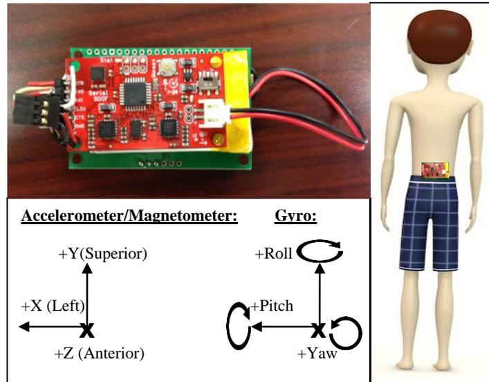
Figure 4-4: Alpha Prototype Orientation
