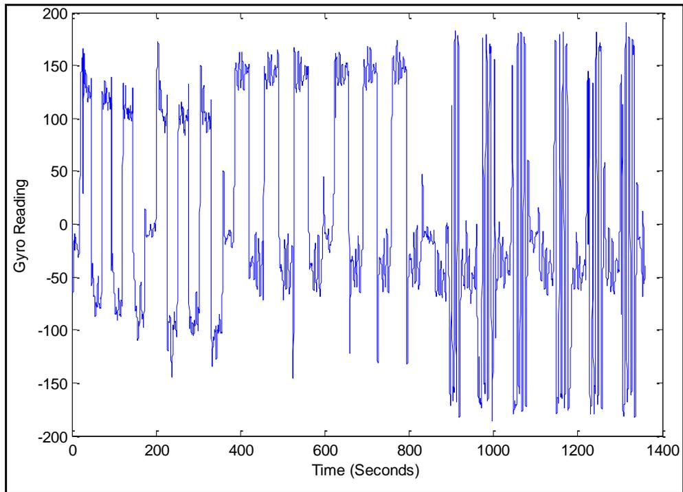
**Figure B-6: Alpha Prototype Gyro Yaw Data (2<sup>nd</sup> Order Butterworth Filter Applied)**
