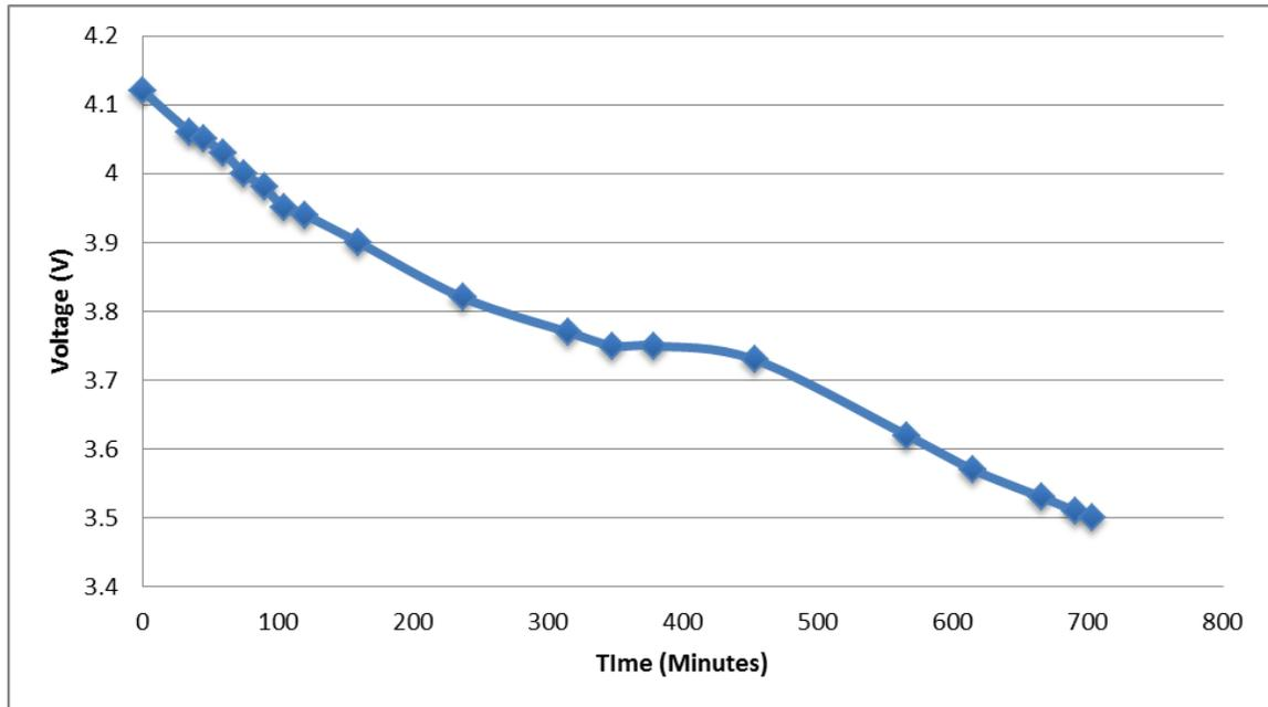
**Figure 5-4: Beta Prototype Voltage Depletion Curve**
