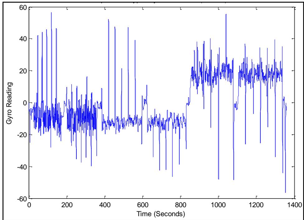
**Figure B-4: Alpha Prototype Gyro Pitch Data (2<sup>nd</sup> Order Butterworth Filter Applied)**
