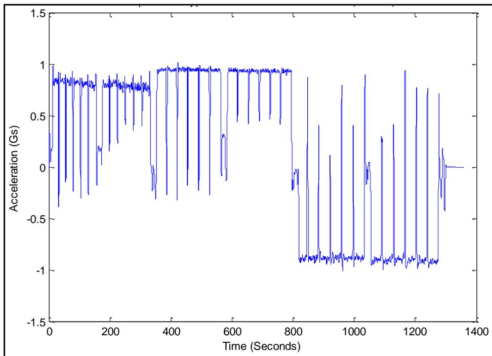
**Figure B-3: Alpha Prototype Z-Axis Accelerometer Data (2<sup>nd</sup> Order Butterworth Filter Applied)**
