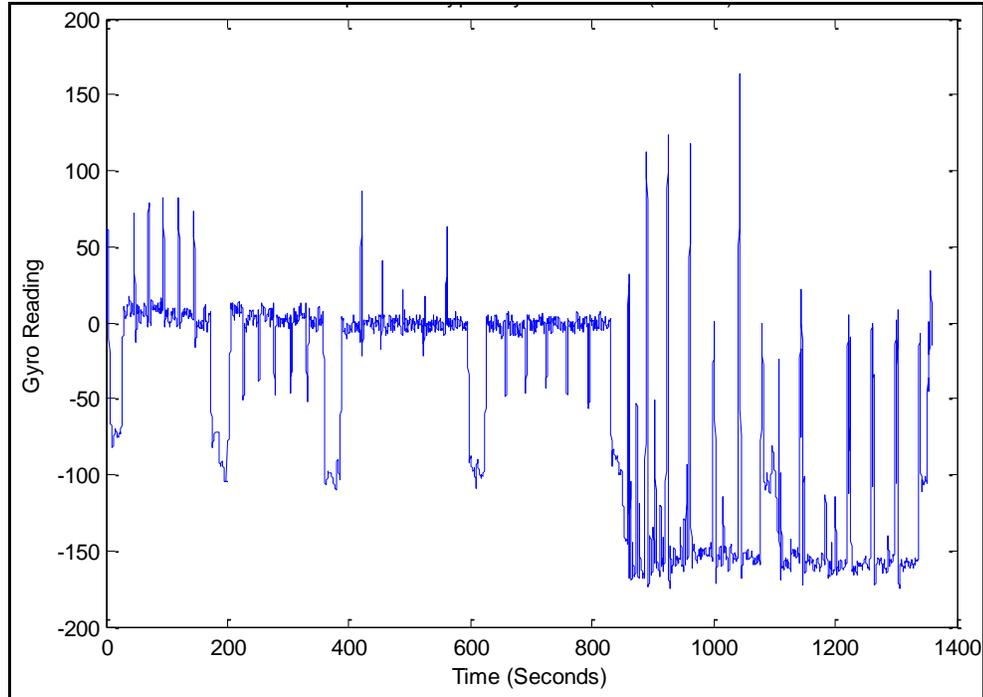
**Figure 5-3: Alpha Prototype Gyro Roll Data (2<sup>nd</sup> Order Butterworth Filter Applied)**
