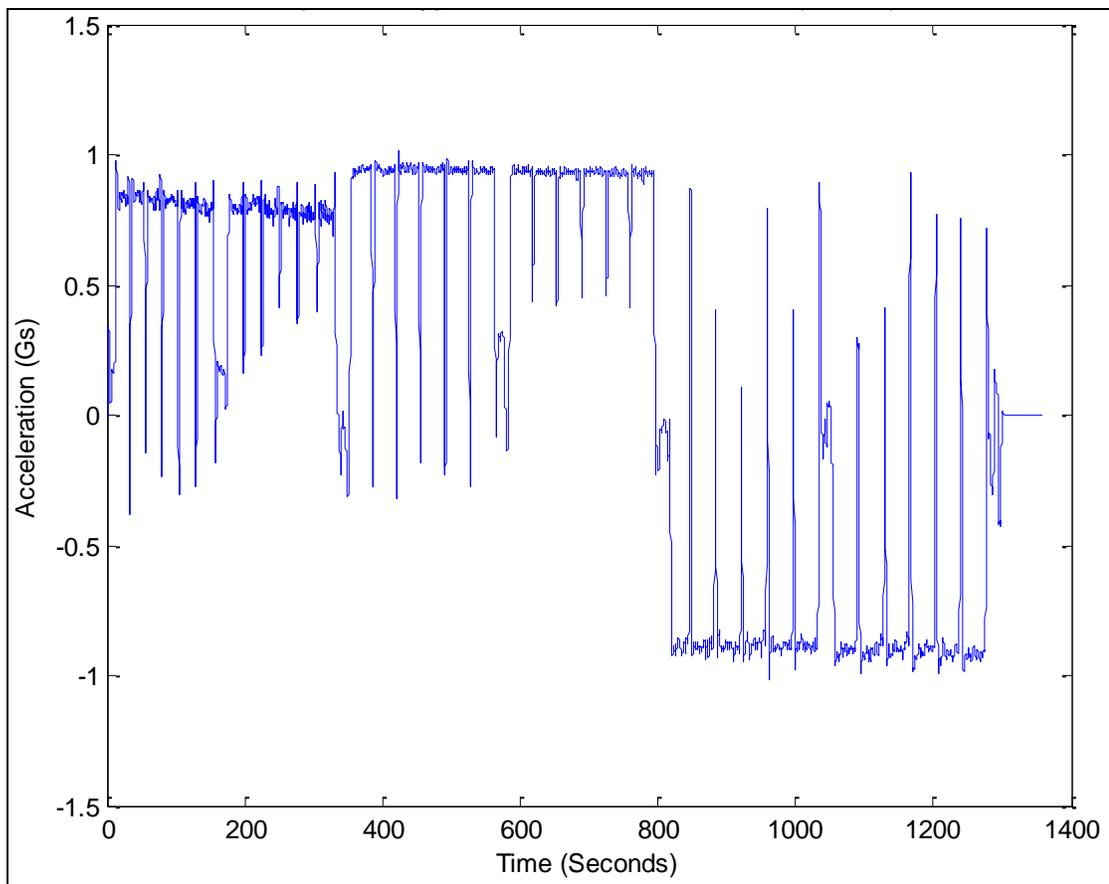
Figure 5-1: Alpha Prototype Test Results (Z-Axis Acceleration, 2<sup>nd</sup> Order Butterworth Filter Applied to Data)
