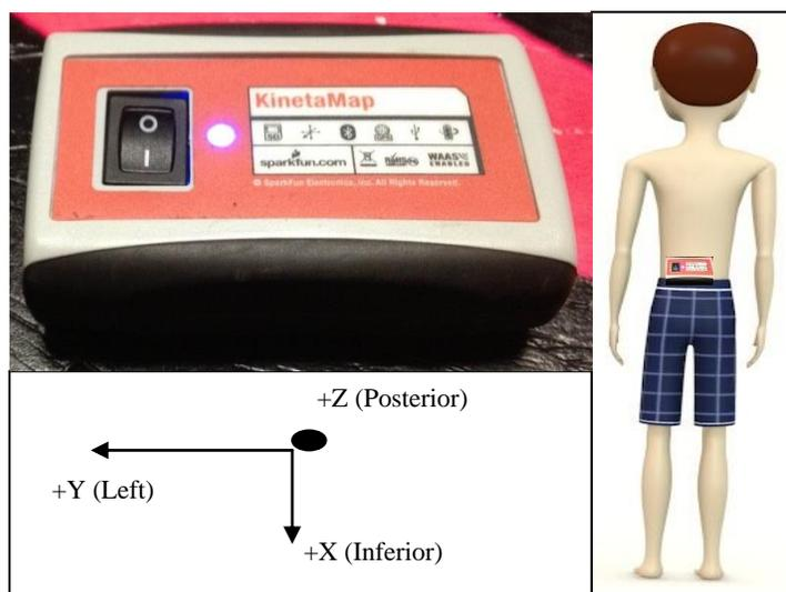
**Figure 4-1: KinetaMap Device Orientation**
