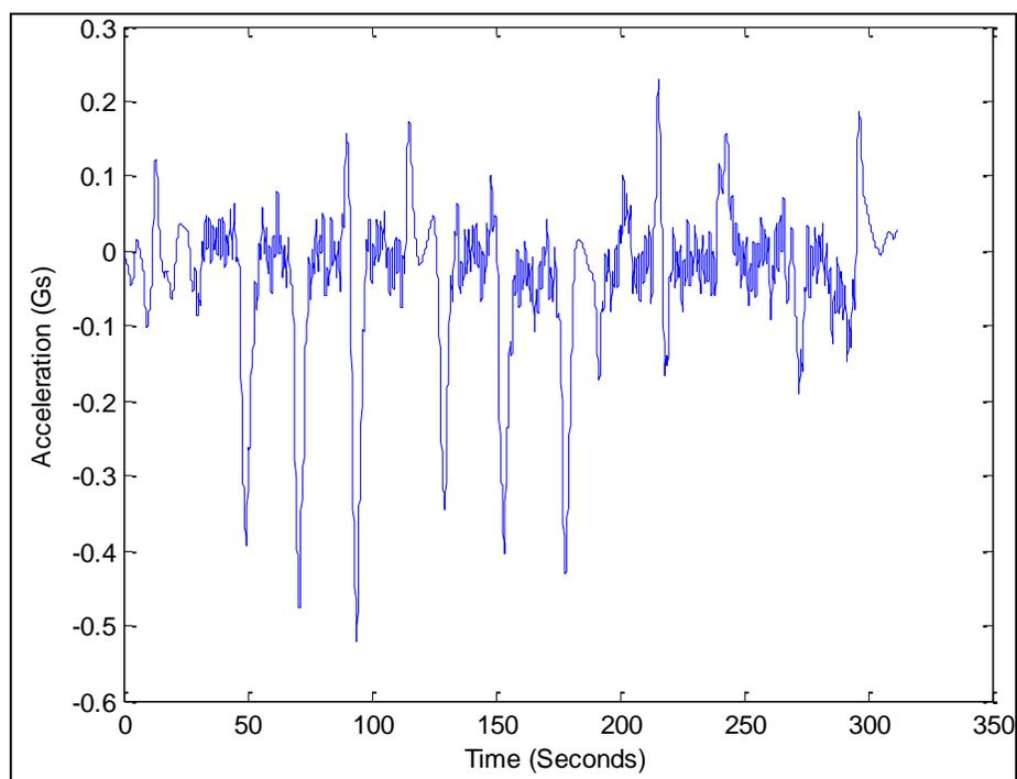
**Figure A-2: KinetaMap Y-Axis Data (2<sup>nd</sup> Order Butterworth Filter Applied)**
