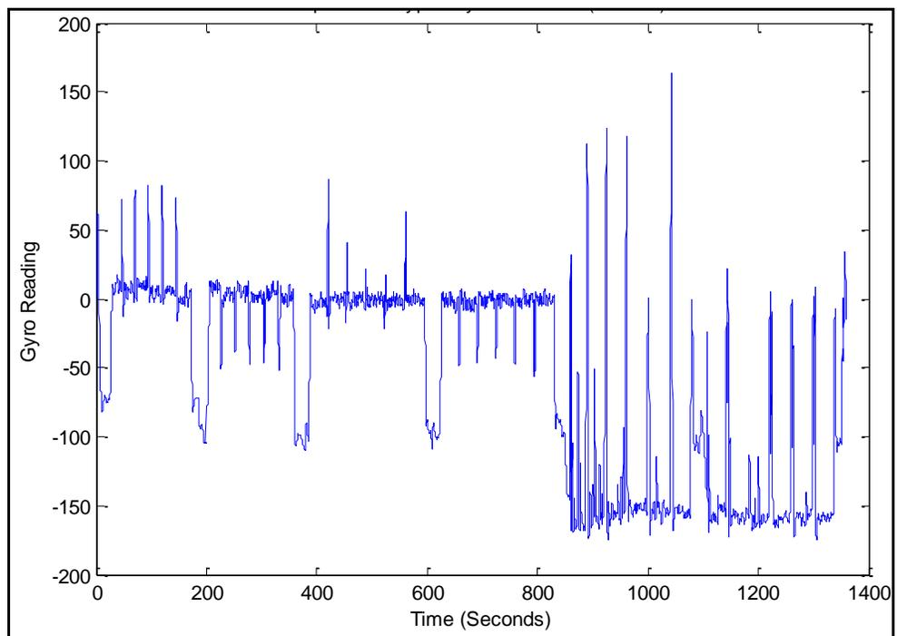
**Figure B-5: Alpha Prototype Gyro Roll Data (2<sup>nd</sup> Order Butterworth Filter Applied)**
