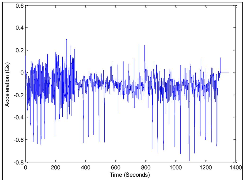
**Figure B-1: Alpha Prototype X-Axis Accelerometer Data (2<sup>nd</sup> Order Butterworth Filter Applied)**
