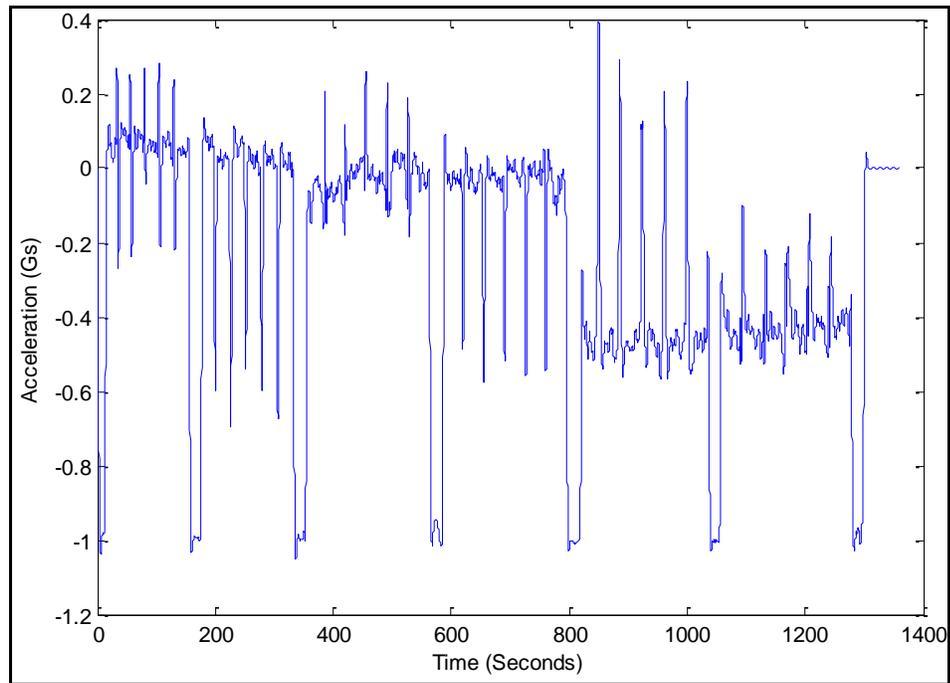
**Figure B-2: Alpha Prototype Y-Axis Accelerometer Data (2<sup>nd</sup> Order Butterworth Filter Applied)**
