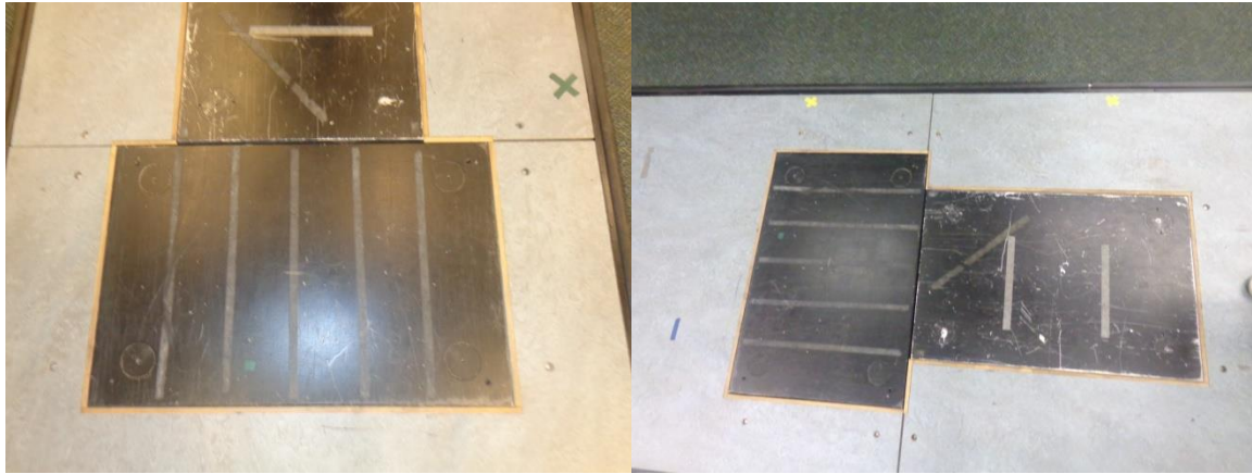
Figure 4 shows the orientation of the two force plates and the tape markers for the curtsy lunge.
