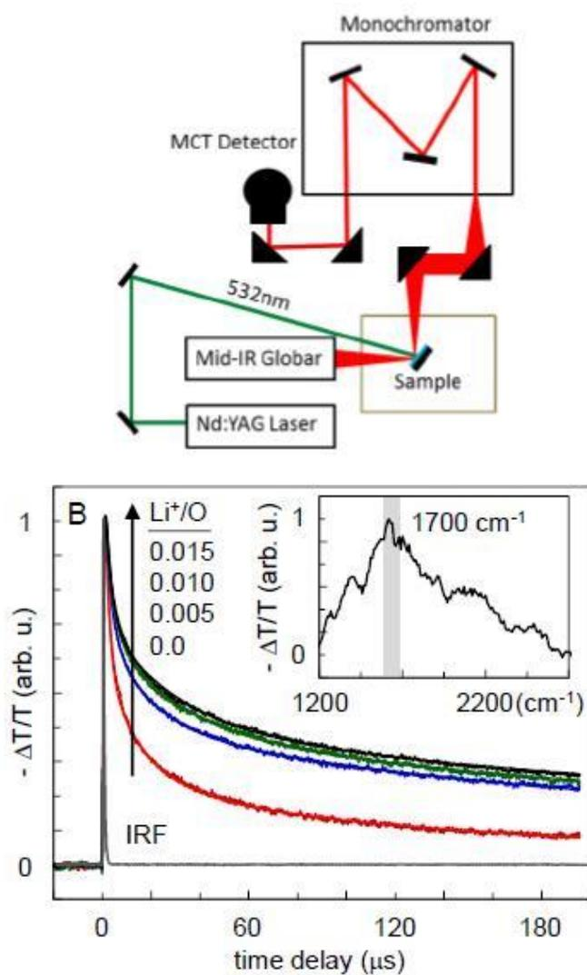
Figure 5-2. Design of the TRIR Instrument Used to Measure Charge Recombination Kinetics and Charge Recombination Kinetics for Various Concentrations of Lithium Ions<sup>y</sup>
