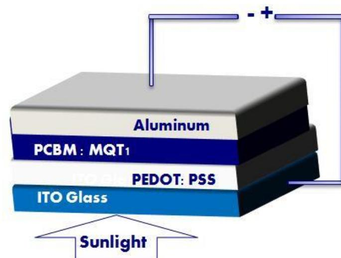
**Figure 2-1. Schematic of a Bulk Heterojunction Photovoltaic Device**
