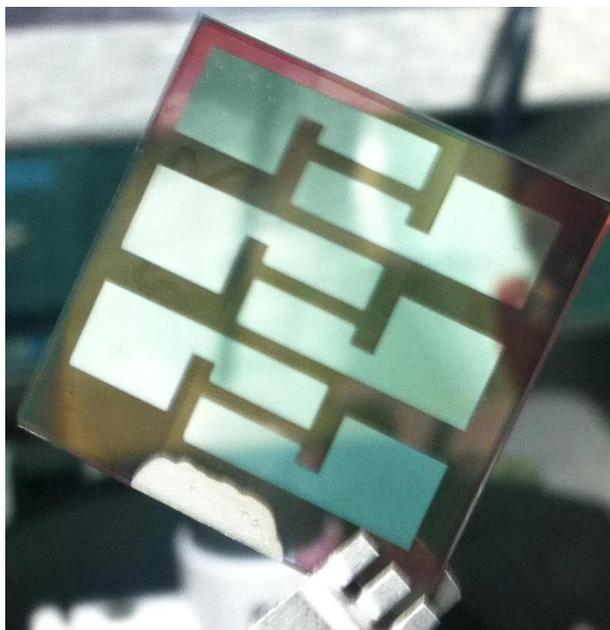
**Figure 3-1. Fabricated Polymer Photovoltaic Device**
