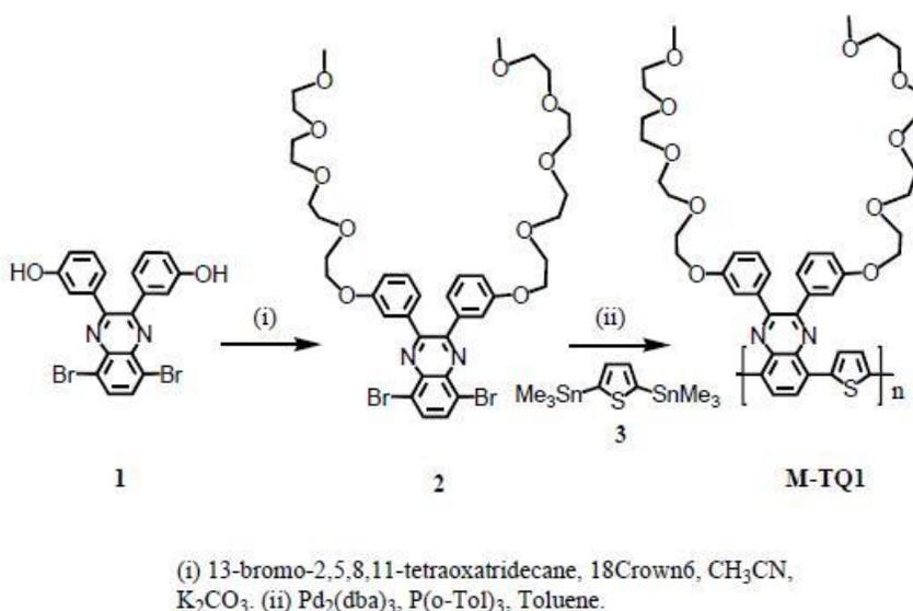
**Figure 2-2. Reaction Mechanism for the Synthesis of M-TQ1**
