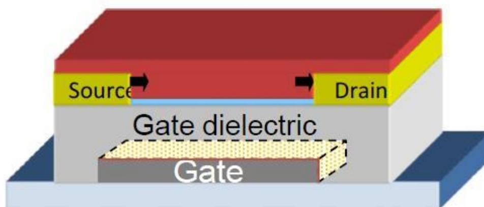
**Figure 4-2. Diagram of a Field-Effect Transistor for Measuring Hole Mobility**
