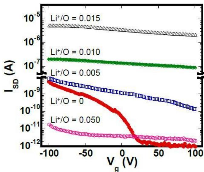
**Figure 4-3. Source Drain Current vs. Gate Voltage for Different M-TQ1 Films**
