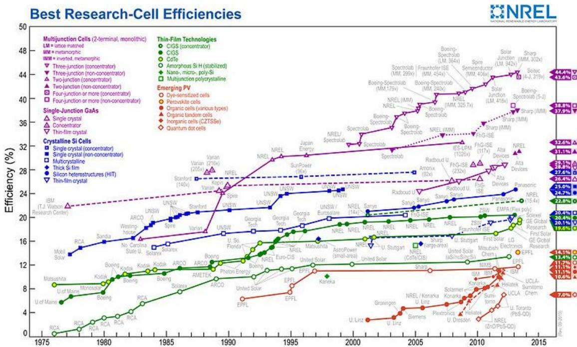
Figure 1-1. Progression of Record Solar Cell Efficiency for Each Type of Technology<sup>6</sup>
