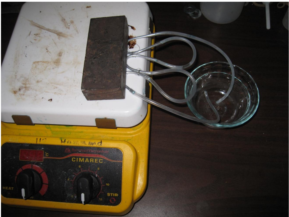
Figure 3.6 – Large Pulsating Heat Pipe setup
