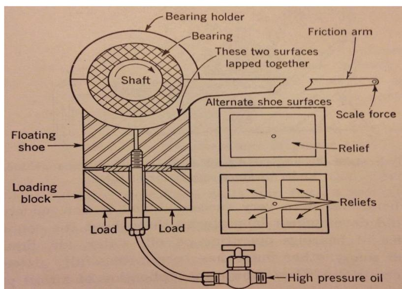
Figure 2. Hydrostatic lubrication as applied to bearing-testing machine. From *Theory and Practice of Lubrication for Engineers* by D. Fuller, 1956, page. 83
