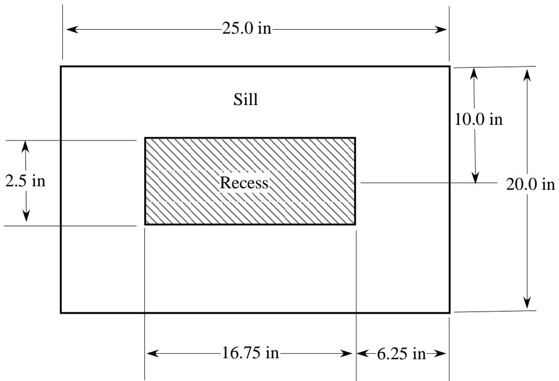
**Figure 7. Schematic of the geometry used in the 2D case (not drawn in scale)**
