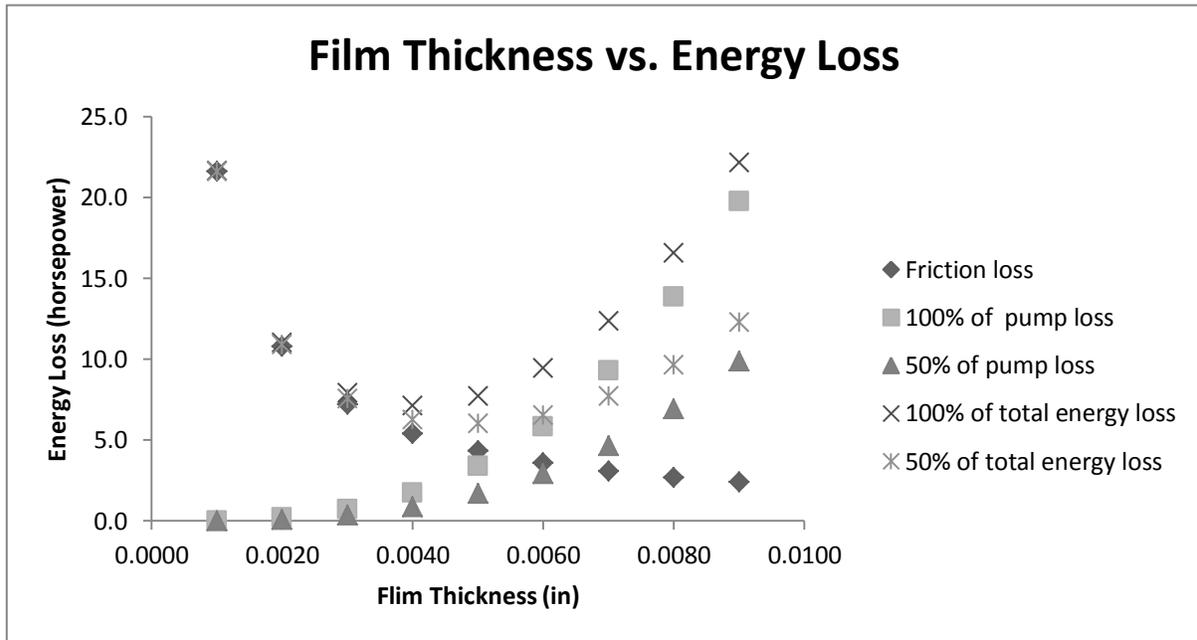
Figure 4. Film thickness vs. energy loss
