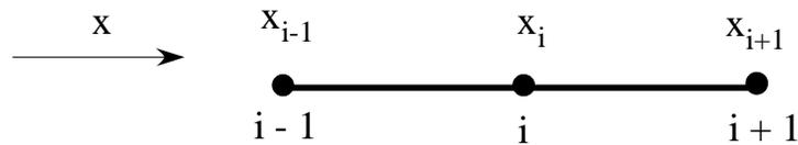
**Figure 5. Schematic of the 1D mesh**
