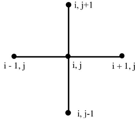
**Figure 9. Schematic of the 2D mesh**
