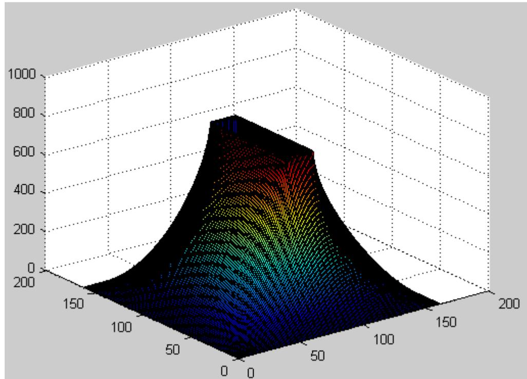
**Figure 10. 2D pressure distribution of the oil pad**
