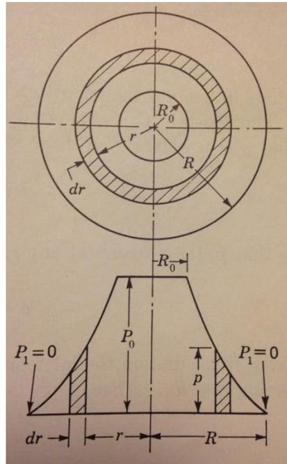
**Figure 3. Plan view and radial pressure distribution of the hydrostatic step bearing. From Theory and Practice of Lubrication for Engineers by D. Fuller, 1956, page. 87**
