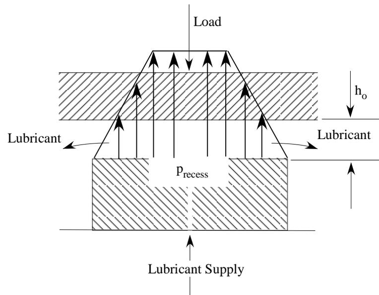
**Figure 1. Schematic of a Bearing in Operation**
