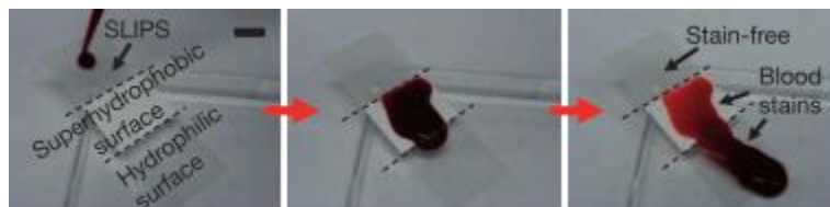
Figure 3: Effectiveness of SLIPS in repelling blood as compared to a superhydrophobic surface and a hydrophilic surface. Reprinted by permission from Macmillan Publishers Ltd: [Nature] (Wong et al.), copyright (2011)
