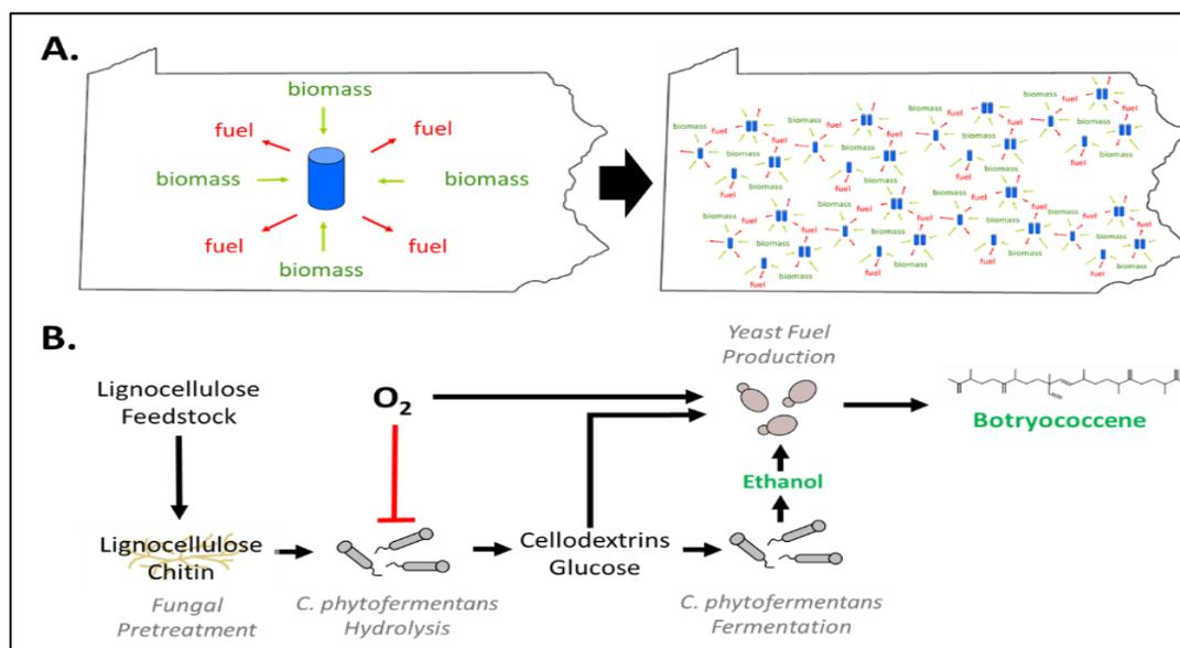
**Figure 1.** FILtH is designed to shift away from traditional, high-cost centralized biorefining toward regional, low-cost biofuels production (A). Hydrocarbon production in FILtH will be achieved through selective bio-pretreatment followed by fermentation using a symbiotic microbial consortium controlled by oxygen transport (B).
