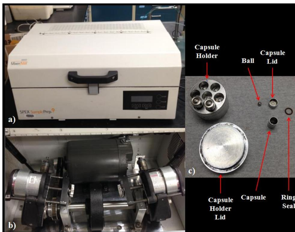
**Figure 17.** An SPEX Sample Prep Mixer/Mill 8000D (a) was loaded with two capsule holders full of samples (b) and grinded down to a homogeneous sample powder. Various parts are necessary for the effective use of this technique (c).
