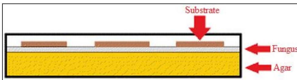
**Figure 13.** Substrate placement technique for SFG sample preparation.
