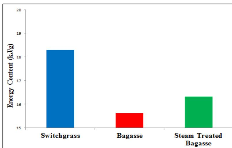
**Figure 24.** Experimental values for the heat of combustion of three different biomass substrates (switchgrass, bagasse, and steam treated bagasse), determined by bomb calorimetry.
