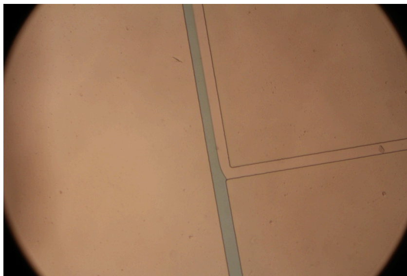
Figure 4. Microfluidic device junction joint between 2 fluid inputs. The blue liquid is flowing in the from the bottom while the clear liquid is flowing in from the right. The 2 then meet at a 90° junction, although they do not mix due to the low Reynolds number.
