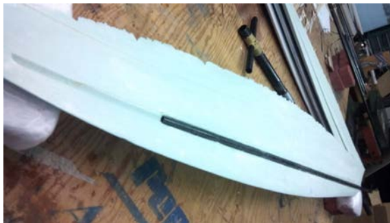
Figure 6-1 Inserting carbon fiber spar
