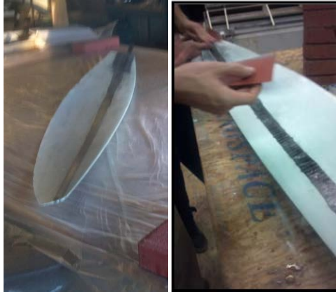
Figure 6-3 Adding carbon fiber strips and sanding
