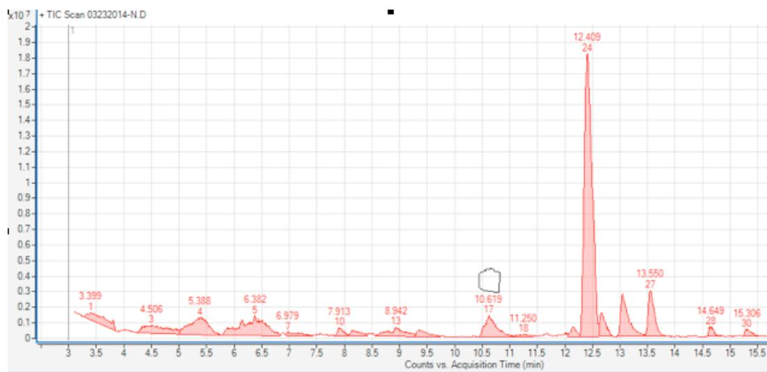
Figure 3-4: Small Batch Sample Chromatogram
