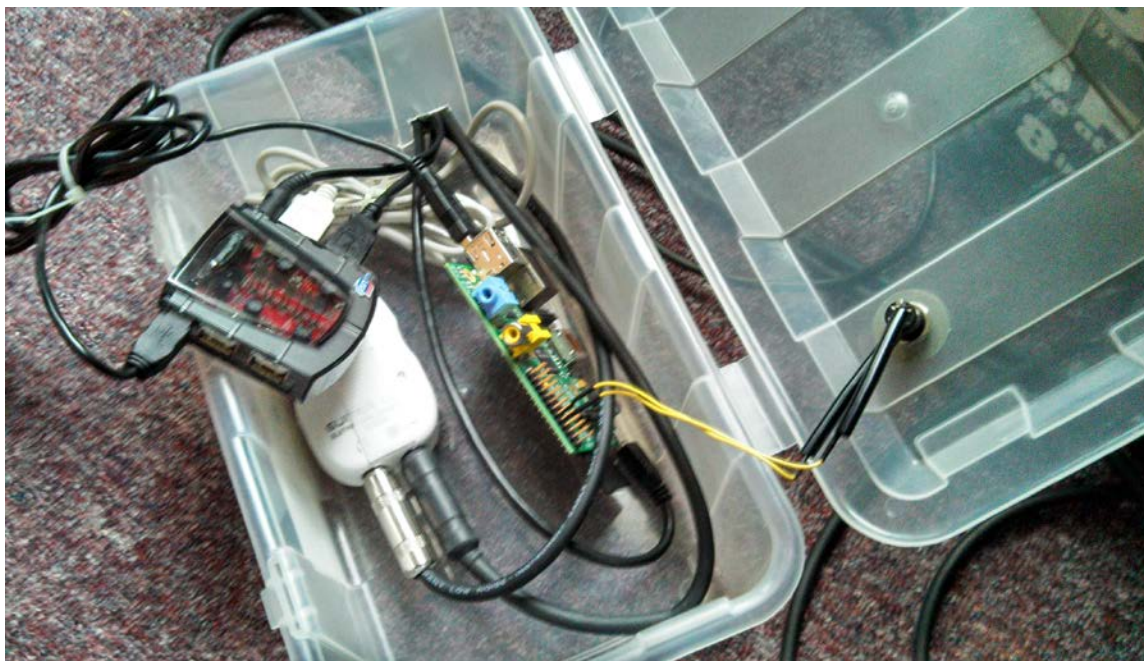
Figure 2: Hardware used in ChainLinkFX – Raspberry Pi (right), Behringer UCG102 (bottom-left), and a Cyberpower USB hub (upper-left)
