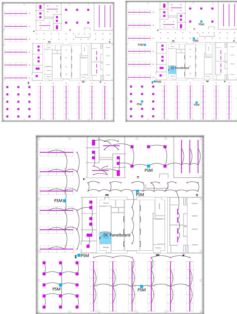
Figure 45: Typical Office Wiring Diagram
