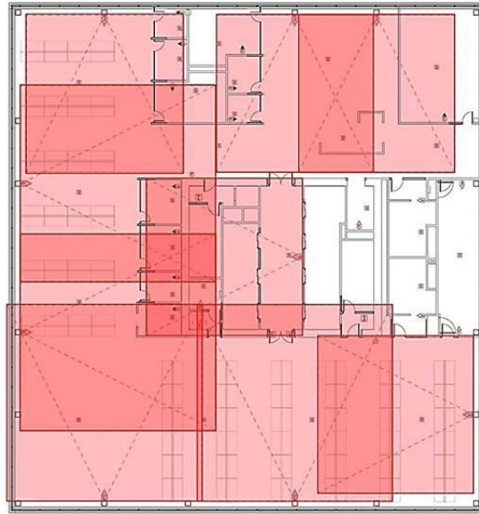
Figure 27: Open Office and Corridor Fire Alarm Annunciation Coverage
