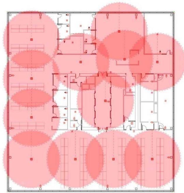
Figure 26: Open Office and Corridor Fire Alarm Smoke Detection Coverage
