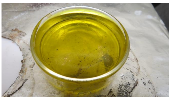
Figure 3.6: Copper foil dissolving in copper etchant
