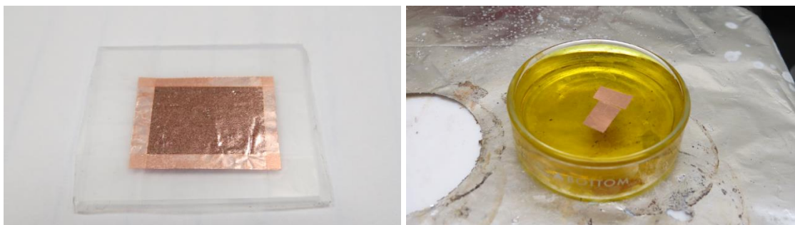
Figure 3.4: Graphene on copper foil, taped on a glass slide Figure 3.5: Copper foil floating on copper etchant
