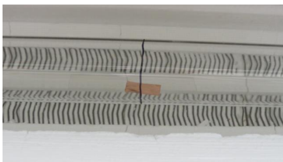
Figure 3.1: Quartz slide, placed in a quartz tube reactor
