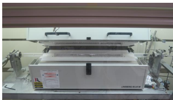
Figure 3.2: Open furnace with copper foil within
