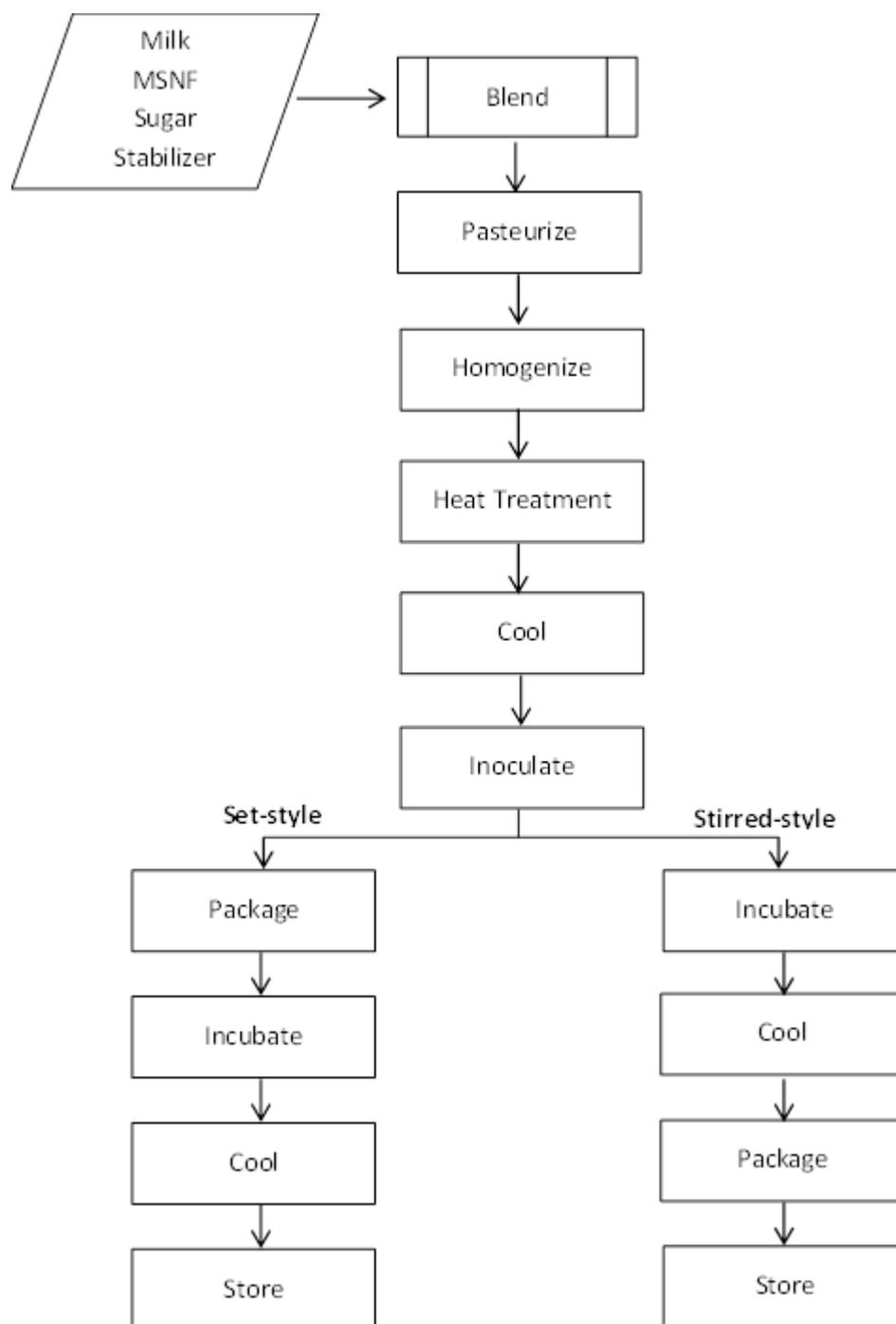
Figure 1-1. Simple Yogurt Processing Flow Diagram (Tamime and Robinson 2007)
