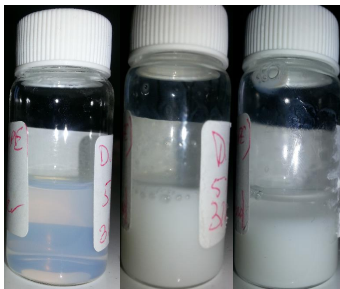
Figure 19: (Sample 2) 5 mL of TMPE-treated silica particles mixed with 5 mL of methanol-water mix. From left to right: before pH change, immediately after pH change, 24 hours after pH change
