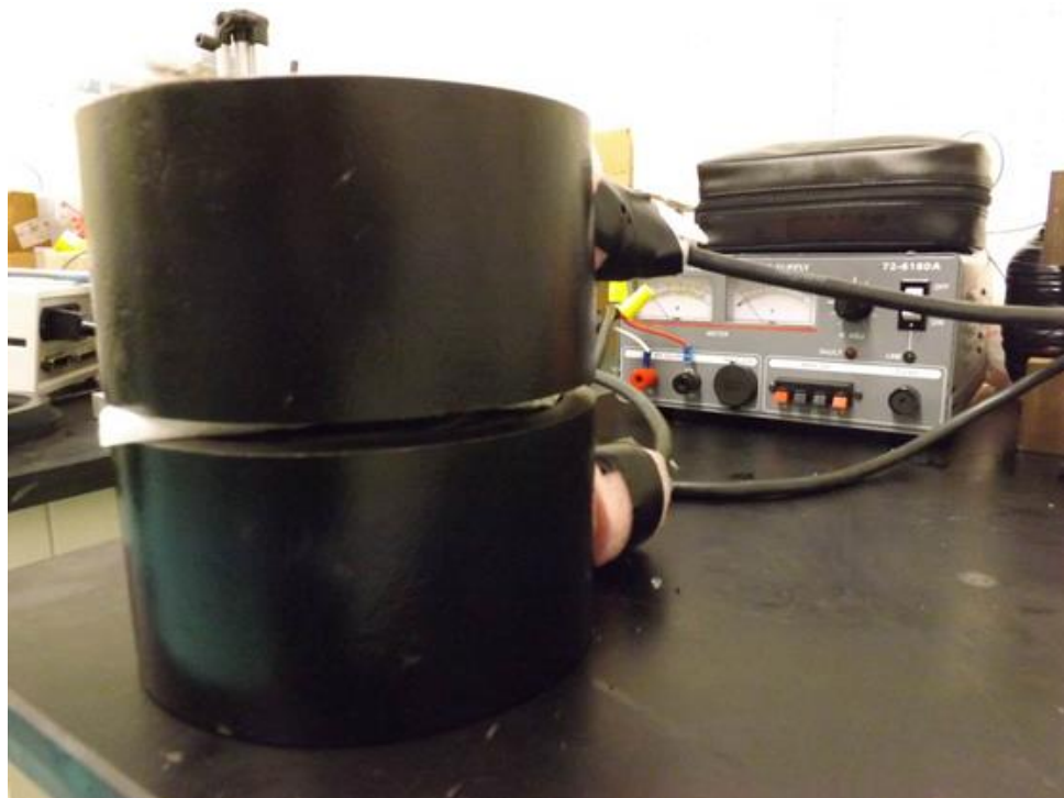
Figure 7. A Magnetech Corp. MFG-6-12 Electromagnet use a 547 kA/m magnetic field to coerce the magnet domains of the MAE into alignment to generate remnant magnetism in the MAE
