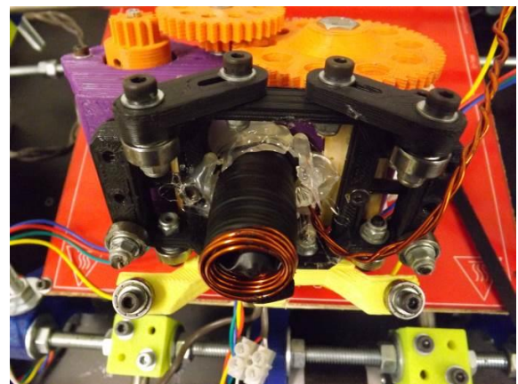
Figure 10. The two layer solenoid wrapped around the syringe is glued to the bottom of the paste extruder
