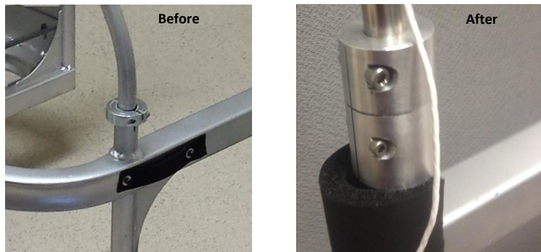
Figure 5: Height adjustment before and after the redesign
