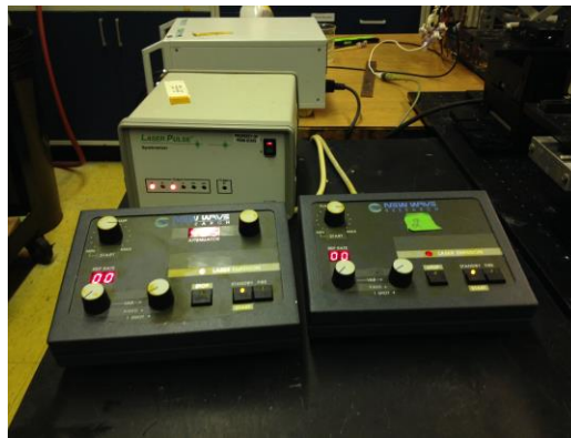
Figure 3-10. Control panels for the two lasers, and the laser synchronizer.
