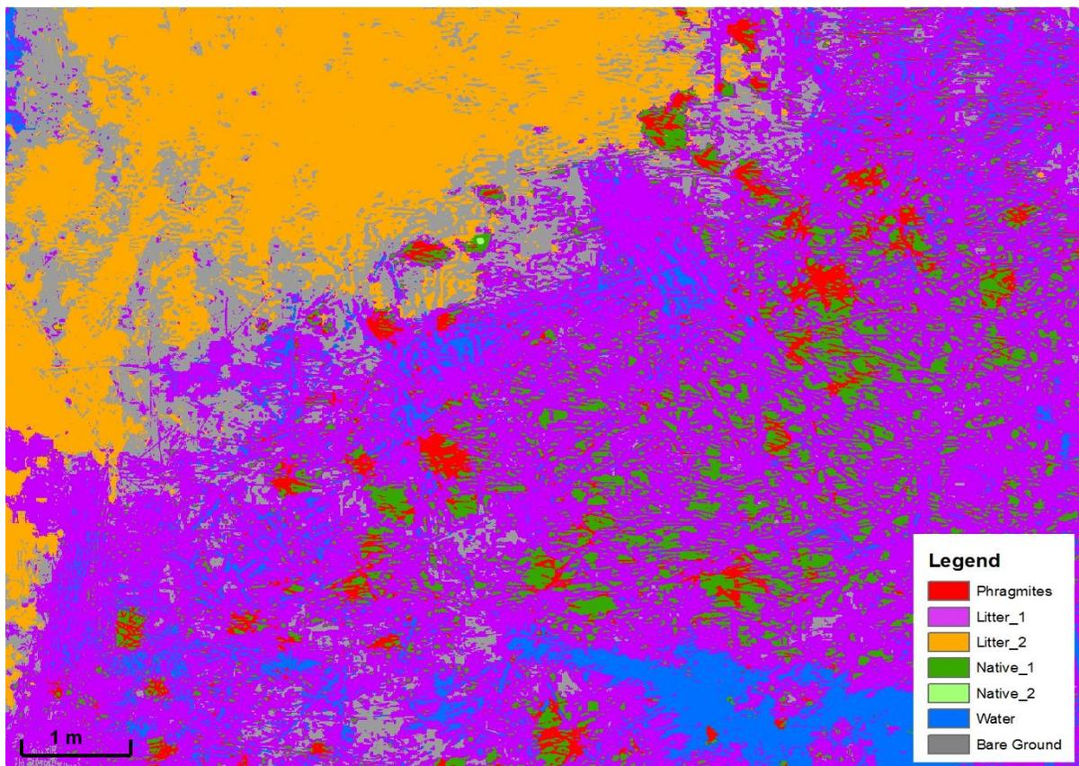
Figure 13. Detail of the classified image mosaic. The small isolated pixels are noise in the classification.
