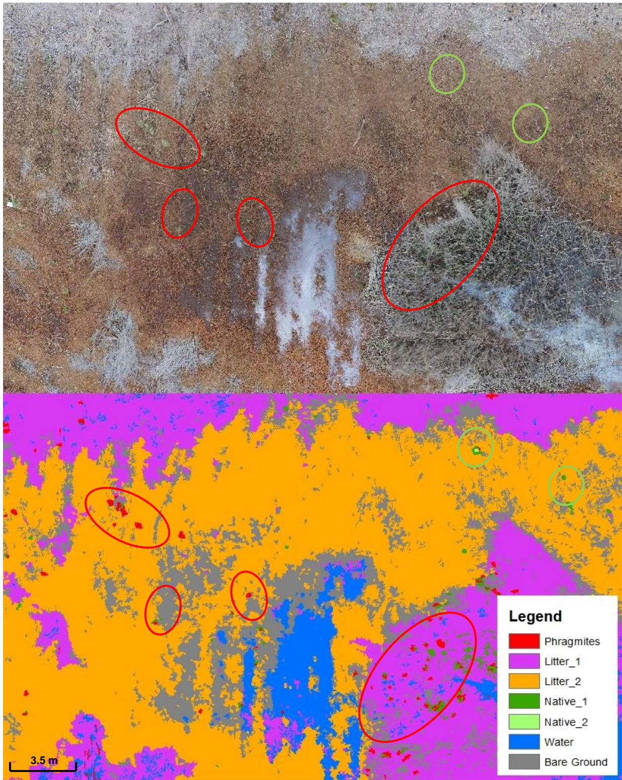
Figure 15. Detail of classified quadcopter-generated mosaic and input image mosaic. Individual *Phragmites* plants are circled in red on the input image mosaic. Native vegetation is circled in green on the input image mosaic.
