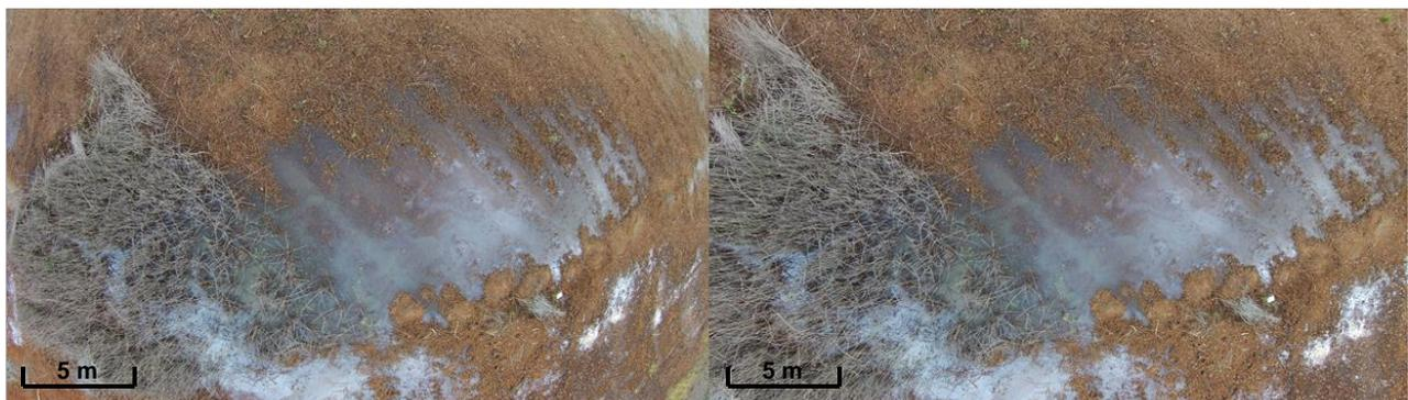
Figure 11. Lens distortion removal in Photoshop CS6. This figure shows one photograph capturing a portion of the study site. The image on the left has not had its lens distortion removed in Photoshop CS6. The image on the right has had its lens distortion removed in Photoshop CS6.
