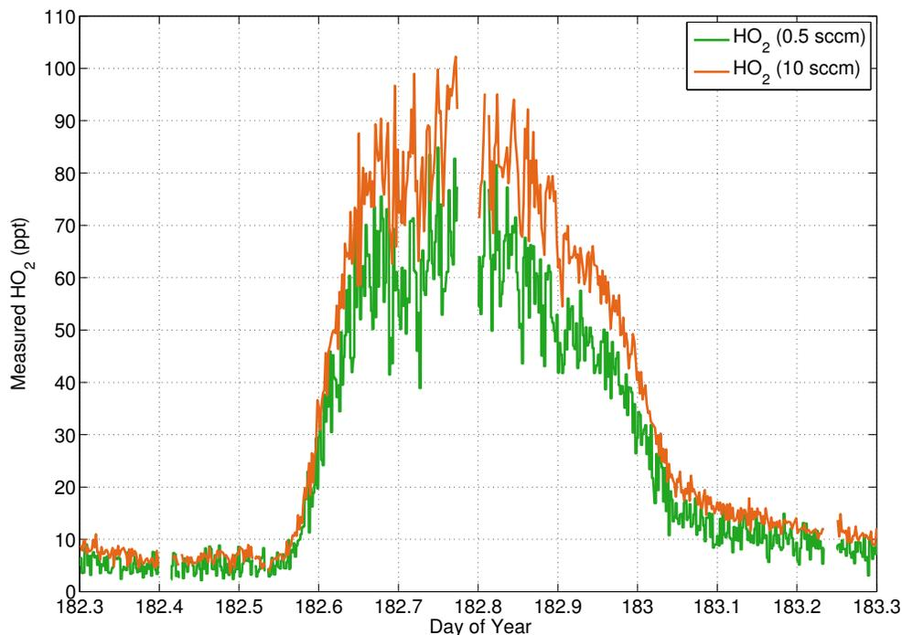
Figure 4.4: HO<sub>2</sub> measurements were greatly affected by RO<sub>2</sub> interference for high NO flows. This is illustrated well in data from July 1. Notice that HO<sub>2</sub> reported by GTHOS is much higher when NO flow into the instrument is 10 sccm.
