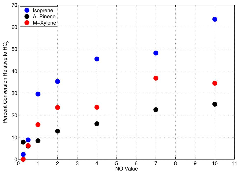
Figure 3.3: Results of the  $\text{RO}_2$  interference testing. While the shape of the conversion curves were similar for all of the gases tested, Isoprene conversion had the largest relative magnitude of the potential  $\text{RO}_2$  sources. Given its large contribution to SOAS  $\text{RO}_2$ , the isoprene conversion efficiencies shown here were used to estimate the  $\text{HO}_2$   $\text{RO}_2$  interference seen during SOAS.
