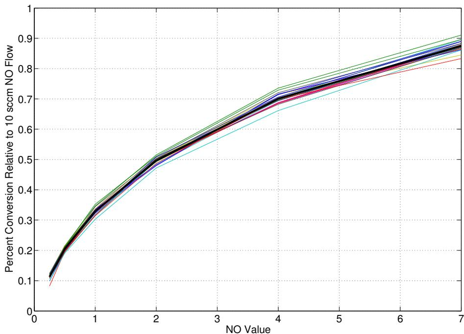
Figure 3.2: Results of the  $\text{HO}_2$  conversion tests performed after SOAS. The conversion efficiency for NO flows relative to 10 sccm flow is shown. GTHOS  $\text{HO}_2$  calibrations are performed with a 10 sccm NO flow. Thus, 10 sccm is used as a reference value to determine measured  $\text{HO}_2$  at lower NO flows.
