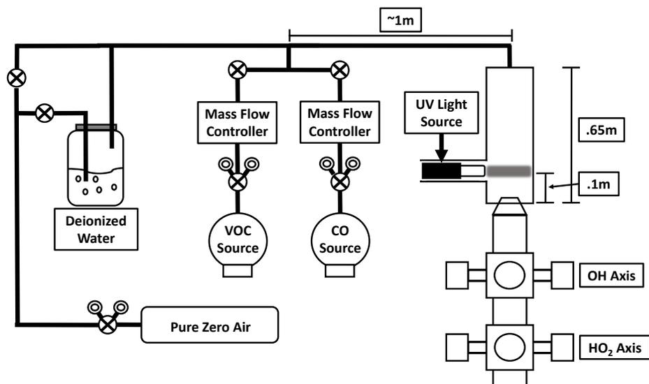
Figure 3.1: Seen here is the setup used to determine the relative signal strength of several common  $\text{RO}_2$ s seen in SOAS. Humidified air flow is modified by the addition of controlled flow of either a CO mixture or an  $\text{RO}_2$  mixture. The combined airflow is passed by a mercury lamp to create a large OH signal which reacts with the other present gas species as they enter the instrument.
