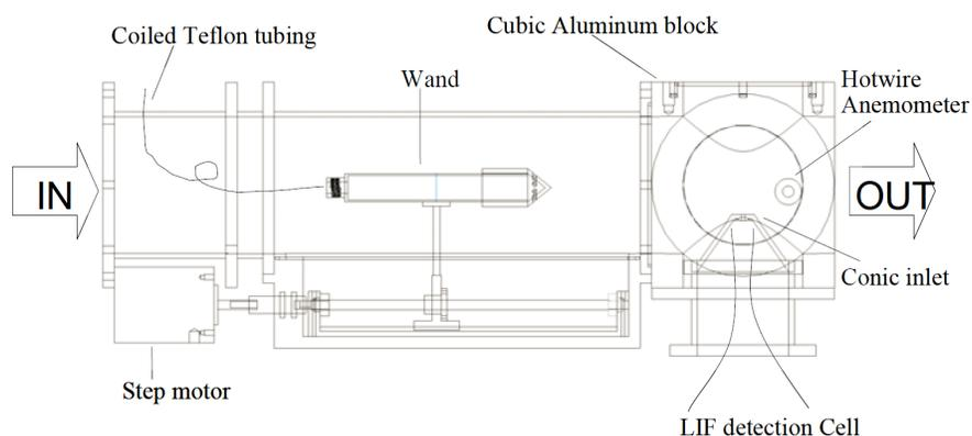
Figure 2.2: This schematic diagram shows a cross section of The OH reactivity instrument setup as it was used to take measurements during SOAS. Ambient air flows through the main tube while a movable OH source adds copious OH to the flow. The resulting OH signal is measured at the end of the tube and the difference in signal based on the location of the OH source can be used to determine OH reactivity. Figure from Mao et al. (2009).
