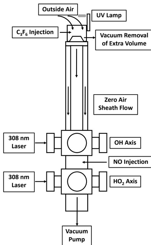
Figure 2.1: This schematic diagram shows a cross section of GTHOS setup as it was used to take measurements during SOAS.  $C_3F_6$  was injected through six 0.25 mm needles which were pointed towards the center of the inlet. Attached just above the inlet was a mercury lamp used for daily testing of the  $C_3F_6$  injection system's effectiveness.
