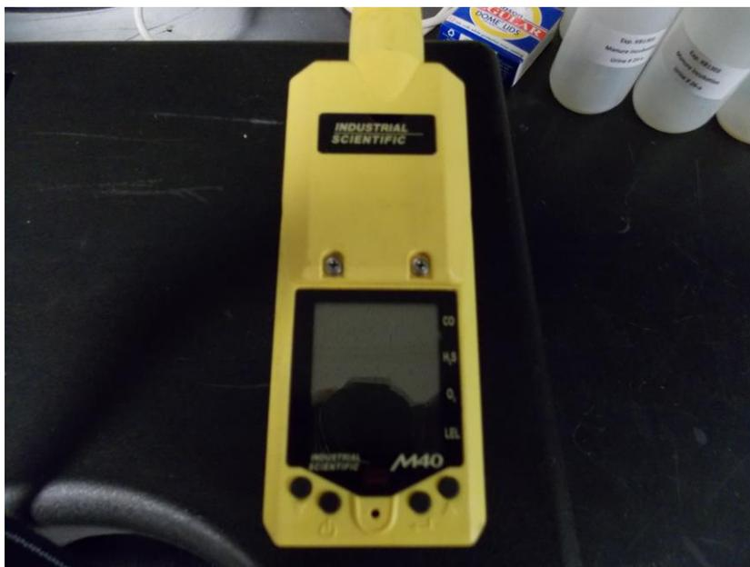
**Figure 4: Industrial Scientific M40 Multi-gas meter**
