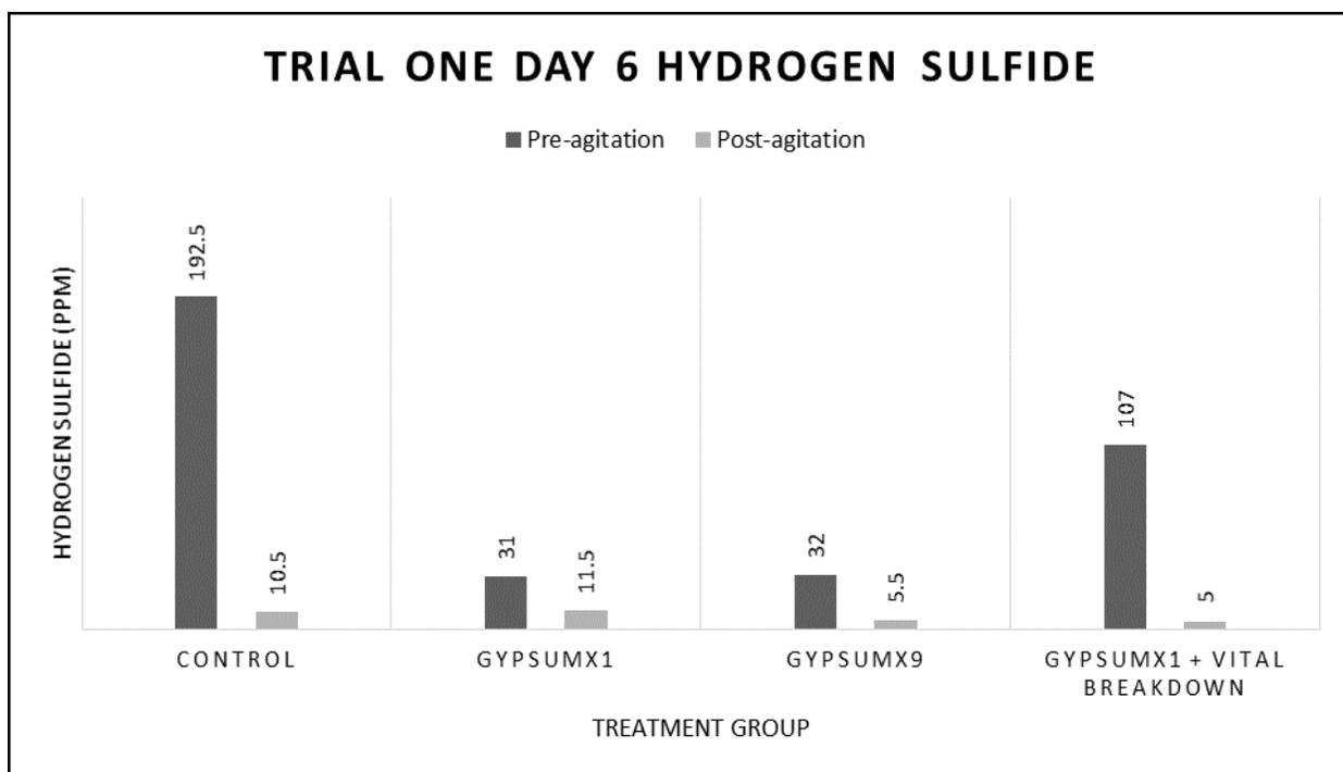
Figure 6: Trial One Day 6 Hydrogen Sulfide
