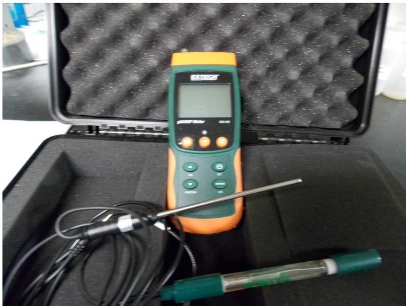
Figure 5: Extech SDL100 pH/ORP/Temperature meter
