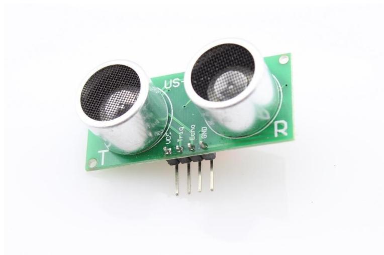
**Figure 2: Image of the Ultrasonic Distance Sensor**
