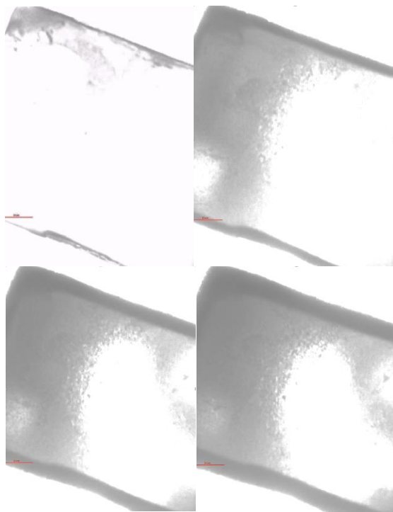
Figure 4. Time-lapse image of KBr crystal replacing in batch reactor with saturated KCl solution. The dark rim represents the newly formed K(Br,Cl) product phase.
