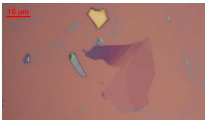
Figure 3-1: Graphene Layer Comparison on SiO 2 , Exfoliated by Zach Zern Oct. 2014
