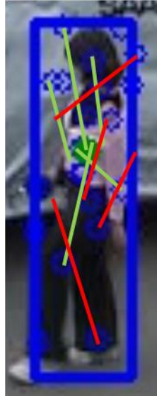
Figure 4. Example of center voting. Green springs are accurate votes for the center while the red springs are votes considered as outliers.
