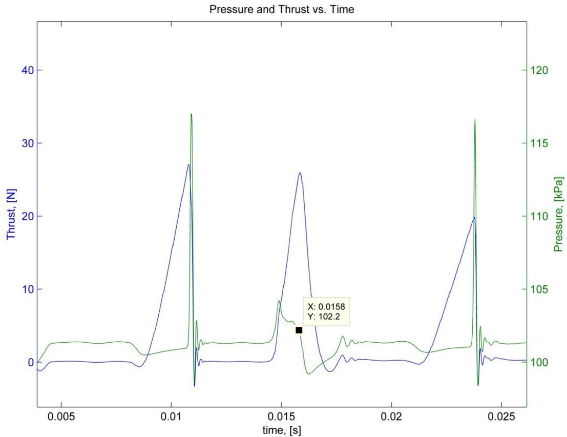
**Figure 9: Pressure Overlay on Thrust**
