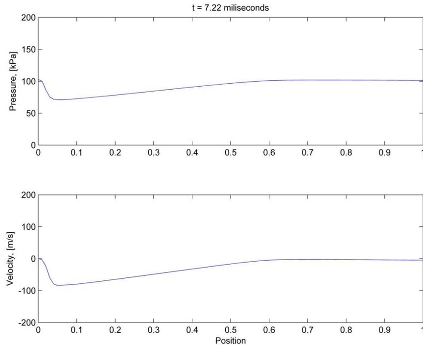
**Figure 7: Flow Velocity Decrease and Backflow in the Combustion Chamber**
