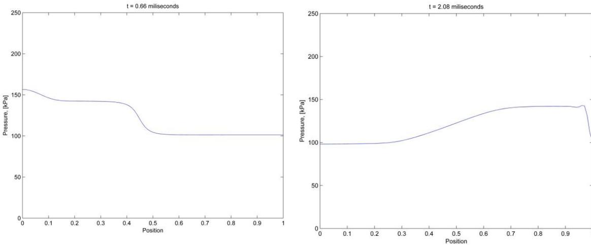
**Figure 3: (Left) Pressure Distribution after Ignition**
