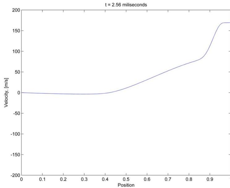
**Figure 6: Velocity Profile when Compression Wave Strikes the Open Boundary**
