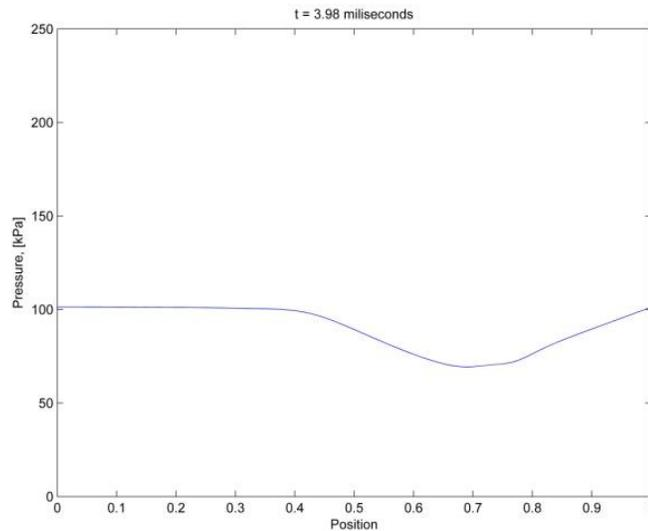
**Figure 5: Reflected Rarefaction Wave**
