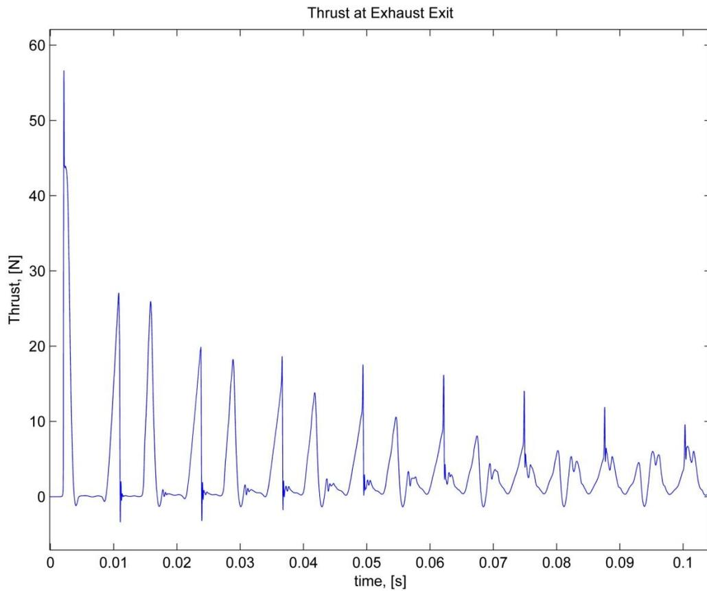
**Figure 8: Thrust Produced by the Pulsejet**
