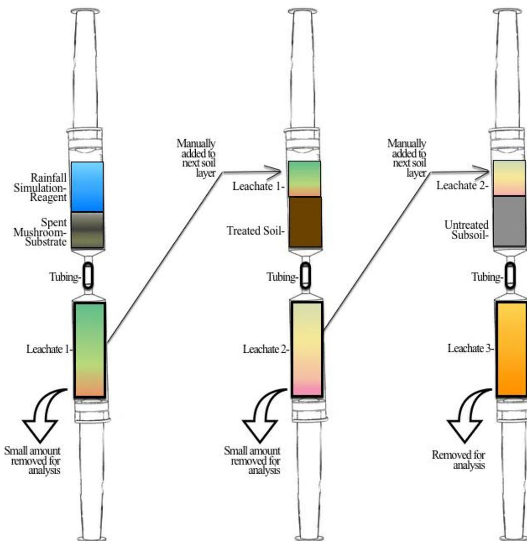
**Figure 2. Segmented soil column schematic in mechanical vacuum extractor. Soil treatments, including manure + paper mill sludge and lime + fertilizer, were compared for P loss and P retention. For experiment one, the soils columns without SMC applied have the first pair of superimposed syringes omitted.**
