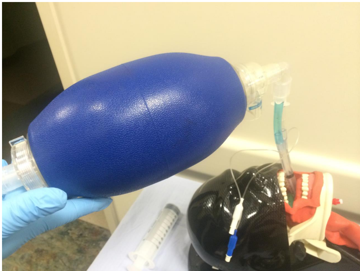
Figure 7. An Ambu bag is connected to the device to determine device placement.
