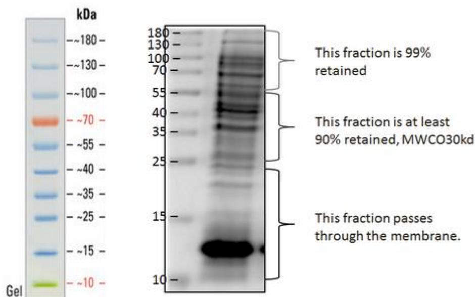
**Figure 15** - SDS gel with corresponding size ladder showing large *E. coli* native proteins (~20-180 kDa) and PLA (~12 kDa). The largest proteins are retained by the membrane very effectively (>55 kDa has 99% retention), while PLA passes through the membrane easily. (Image provided by Tina Lai)
