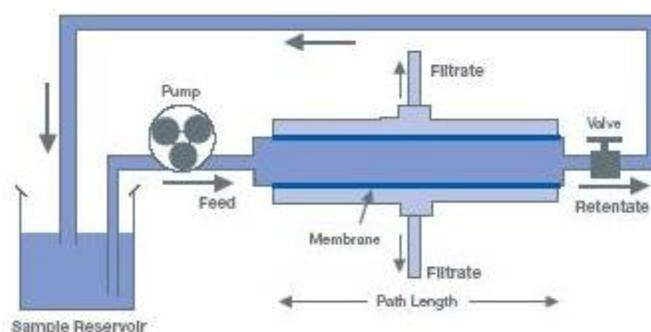
**Figure 14** - Flow path through a simple TFF device. (Taken from Schwartz, Pall Corp., 2015)
