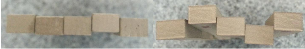
Figure 3 AM tensile specimens as printed standing on end. The photograph on the right highlights the geometric imperfections in one set of end surfaces. Specimen 1 is on the left in both images.
