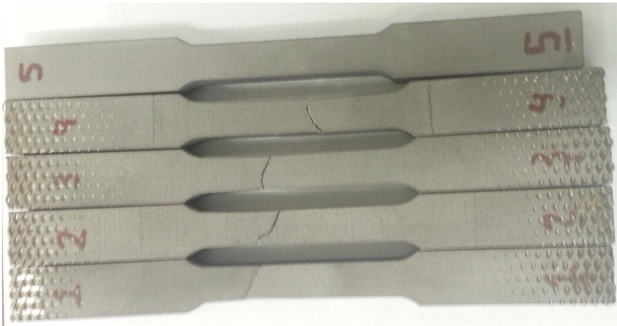
Figure 4 Tensile specimens after fracture. This photograph shows the first 4 failed specimens alongside Specimen 5 before its tensile testing.
