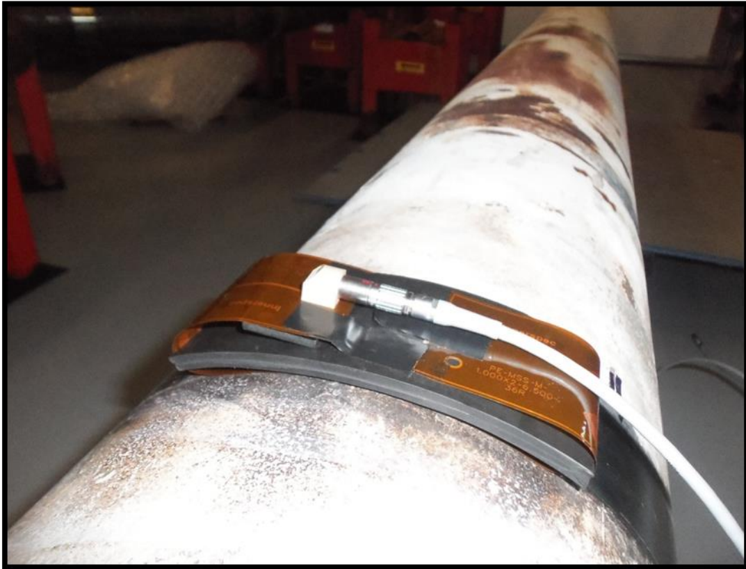
Figure 25: 6.5” length MsS circuit on rubber mount. The MRUT can only accommodate apertures of 3.5 inches or less, so rubber mounts were used for the 6.5” circuits and ribbon cable.
