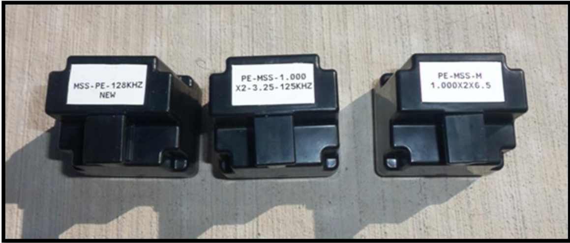
Figure 23: Impedance matching modules for the ribbon cable at 128 kHz, the 3.25” MsS circuit, and the 6.5” MsS circuits.
