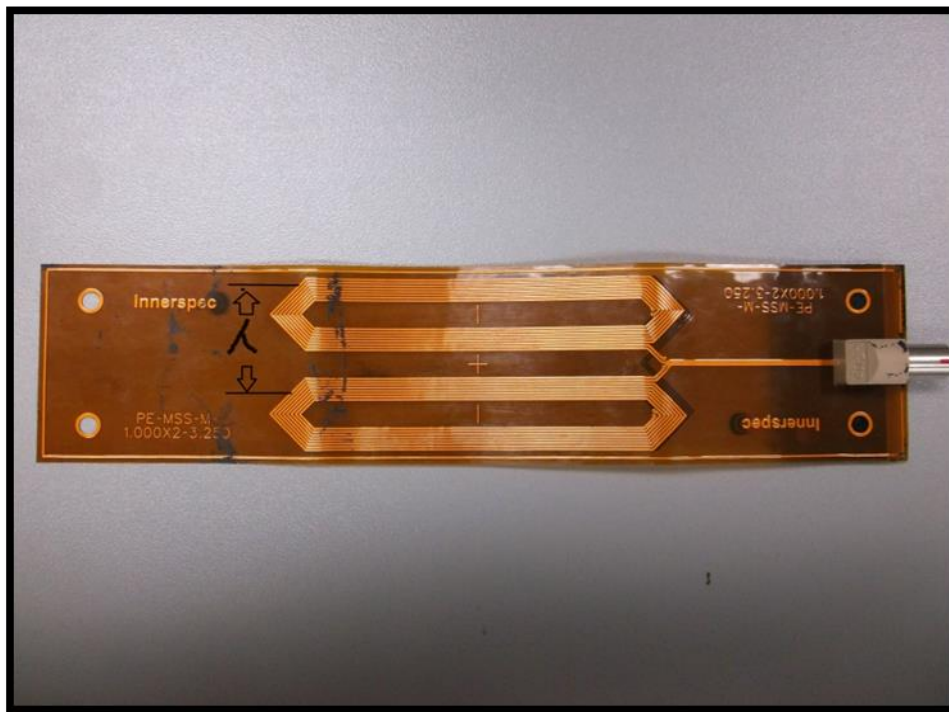
Figure 15: Illustration of finger spacing and wavelength on an MsS circuit type comb transducer.
