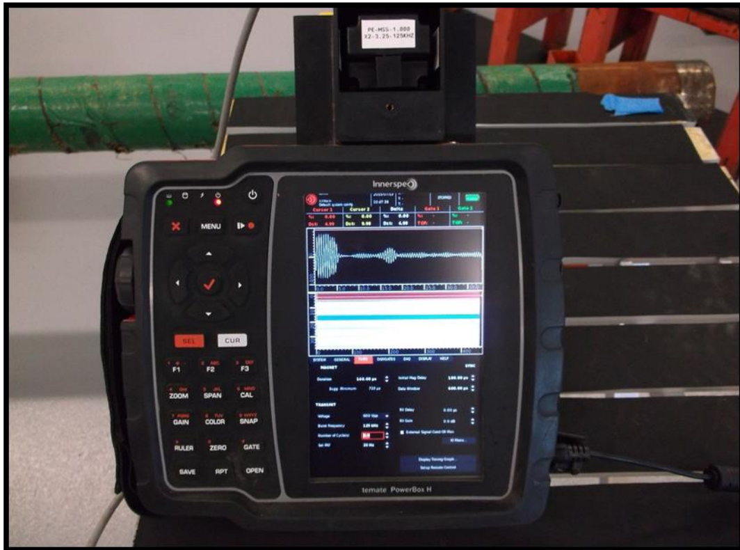
Figure 22: The control panel and display of the Innerspec PowerBox H pulser/receiver. Notice the impedance matching module (with the white sticker) which plugs in just above the display.
