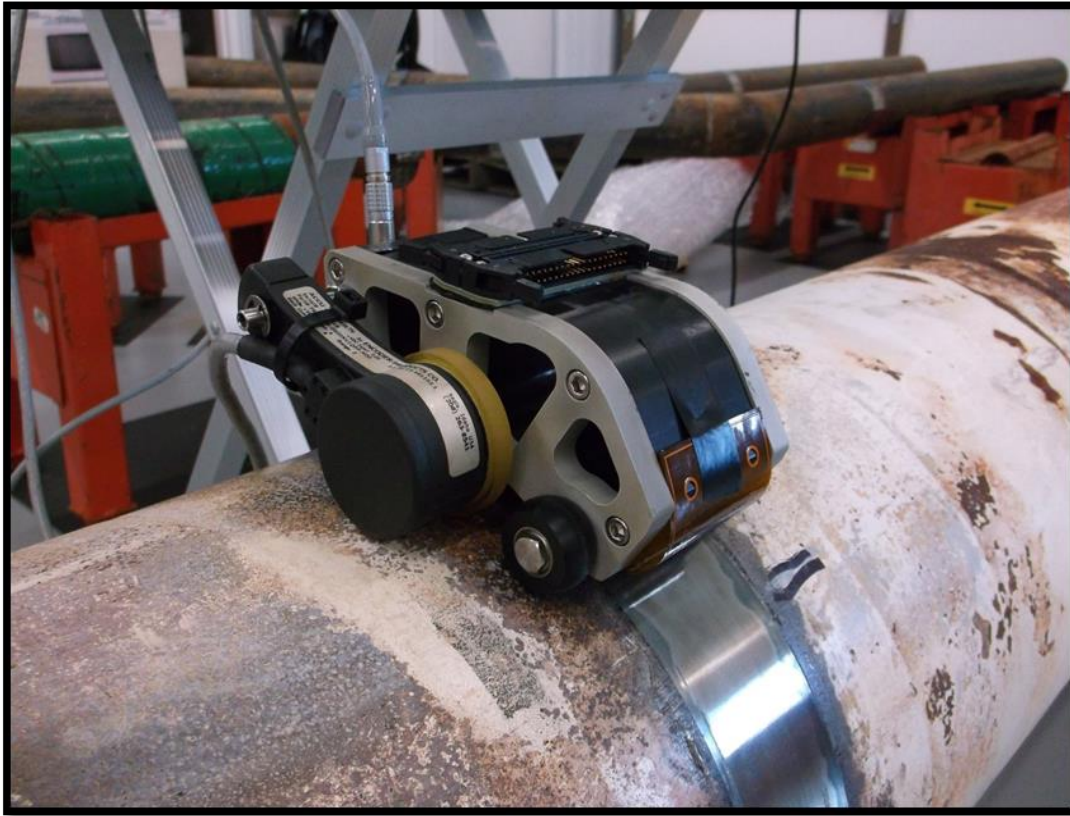
Figure 24: The MRUT probe mounted above a FeCo strip on a 10.5” pipe. The yellow colored wheel on the side of the MRUT is the encoder wheel. A circuit board for attaching ribbon cables is visible on top of the MRUT, but no ribbon cable is plugged in. On the front of the MRUT, an MsS circuit attached with electrical tape is visible.
