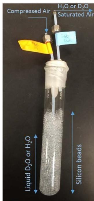
Figure 7: Apparatus for introducing humid environment.
