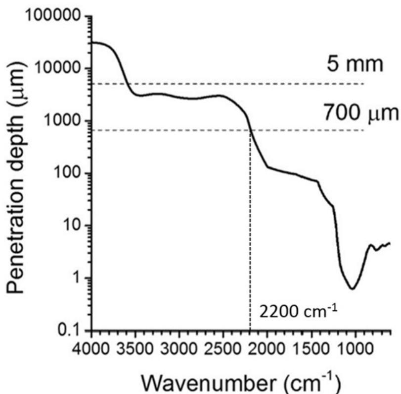
Figure 5: Penetration depth of SR-IR beams in soda-lime glass. Image Credit: Amma et al<sup>14</sup>.
