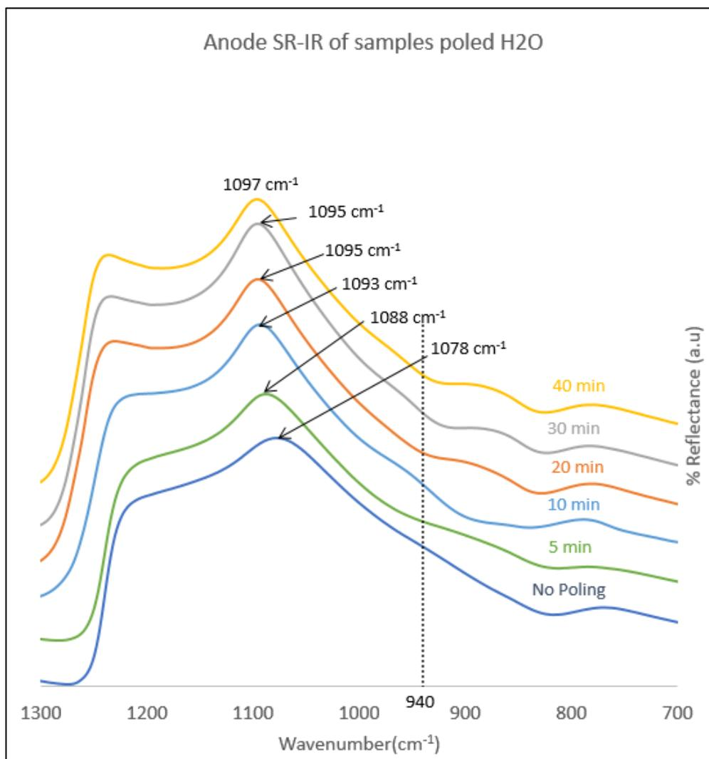
Figure 11: Anode SR-IR spectra of samples poled in a humid environment for 0, 5, 10, 20, 30, and 40 minutes.
