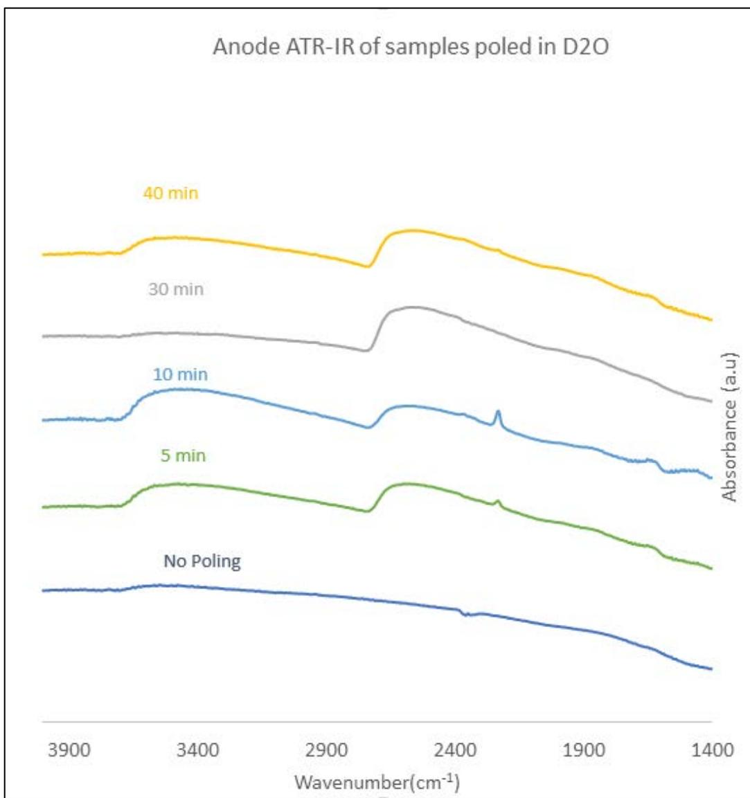
Figure 18: ATR-IR spectra on anode side of samples poled in D2O environment for 0, 5, 10, 30, and 40 minutes. Data Credit: Jiawei Luo.
