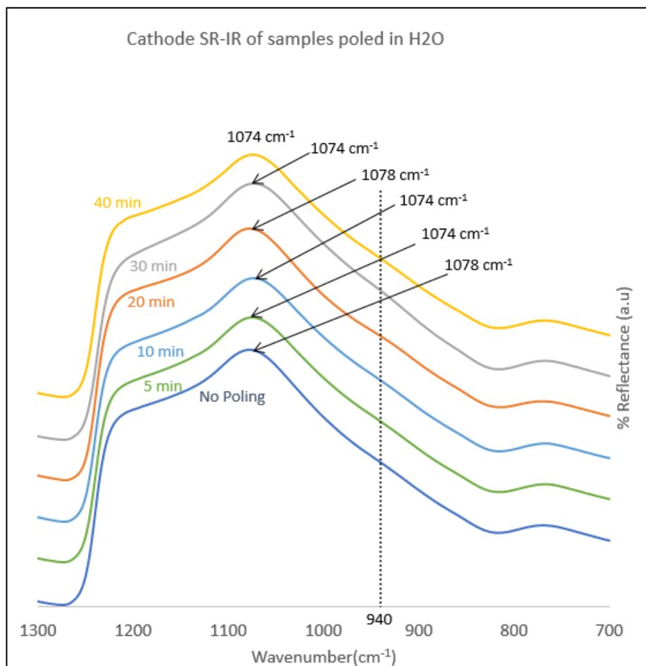
Figure 13: SR-IR spectra of cathode side of glass for different poling times.
