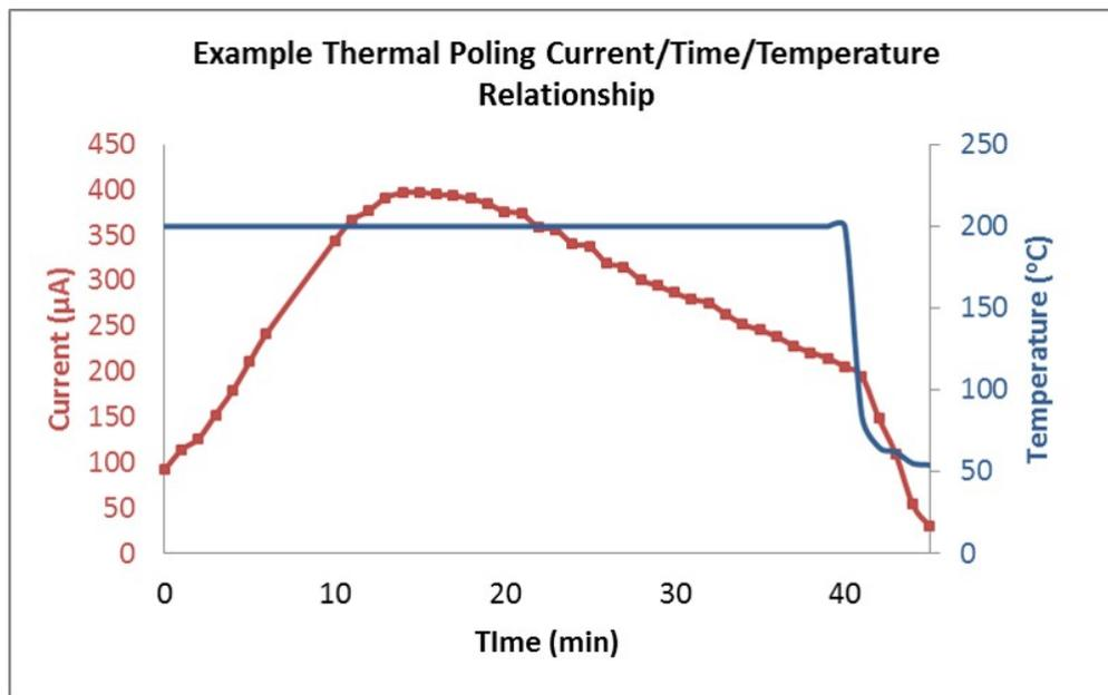
Figure 3: Example current and temperature versus time plot for thermal poling procedure.
