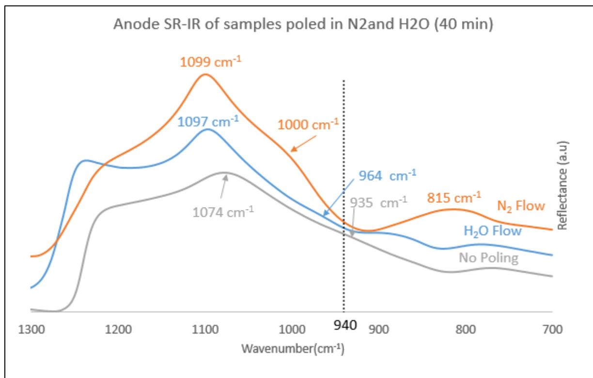
Figure 10: SR-IR spectra of anode side of poled glasses from 700-1300 cm<sup>-1</sup>.
