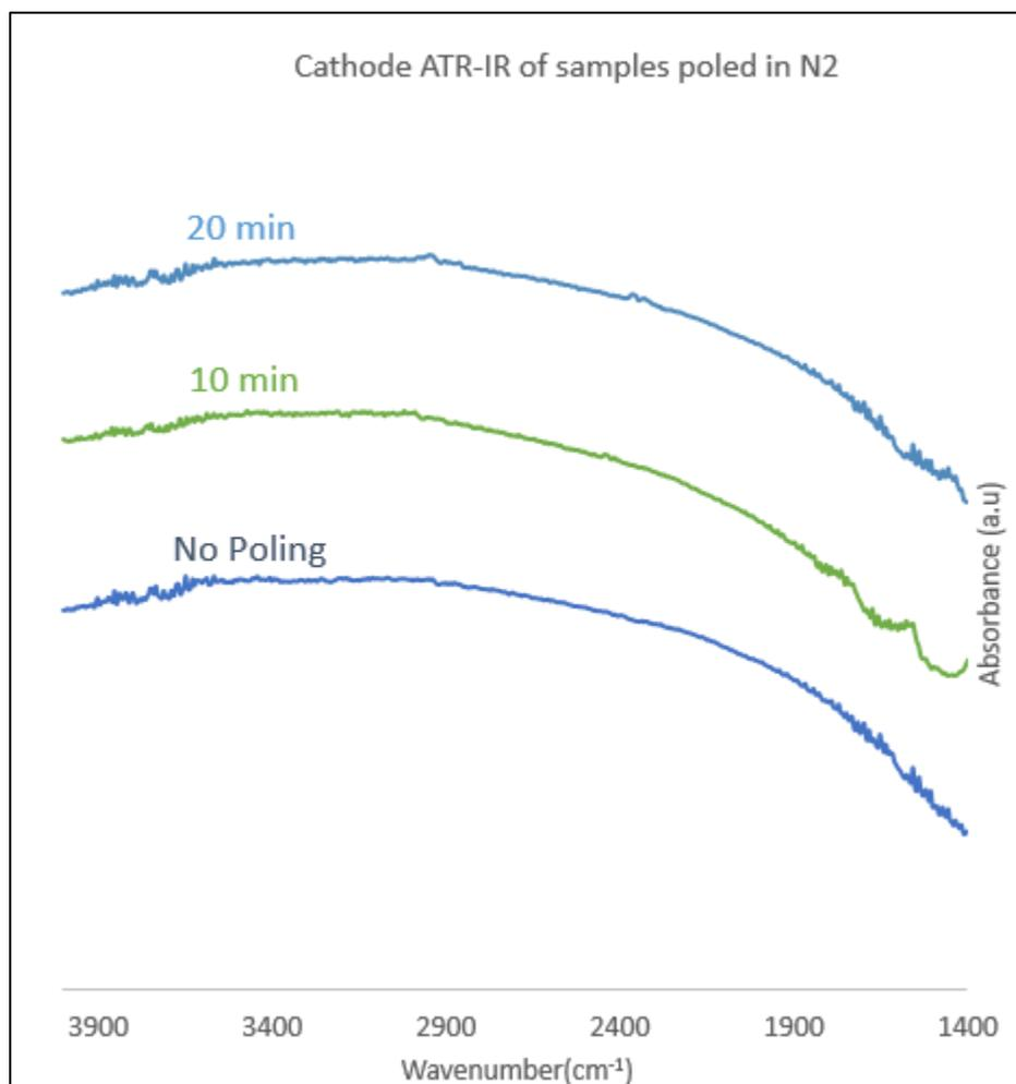
Figure 20: ATR-IR spectra of samples poled in nitrogen environment for 0, 10, and 20 minutes on cathode side. Data Credit: Jiawei Luo
