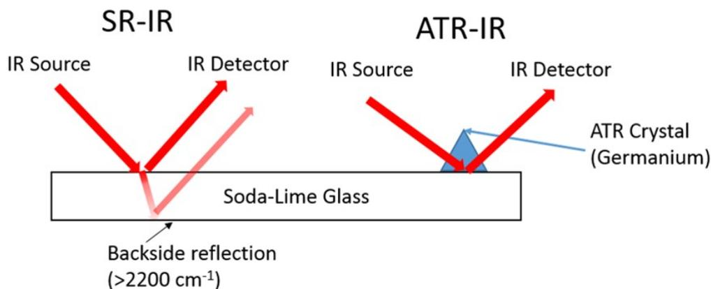
Figure 4: Specular reflection (SR), and attenuated total reflection (ATR) IR techniques.
