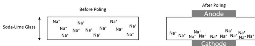
**Figure 1: Sodium ion distribution before and after poling.**
