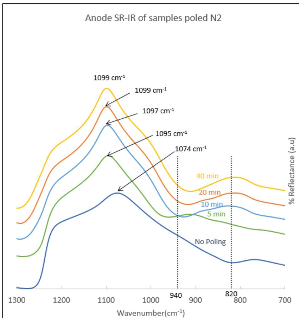
Figure 12: Anode SR-IR of samples poled in a nitrogen environment for 0, 5, 10, 20, and 40 minutes. Data Credit: Jiawei Luo.
