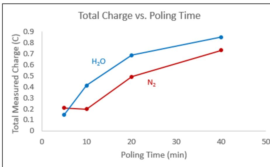
Figure 9: Total measured charge versus poling time for samples poled in humid and inert environments.
