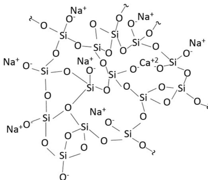
Figure 2: Example chemical structure of soda-lime glass.
