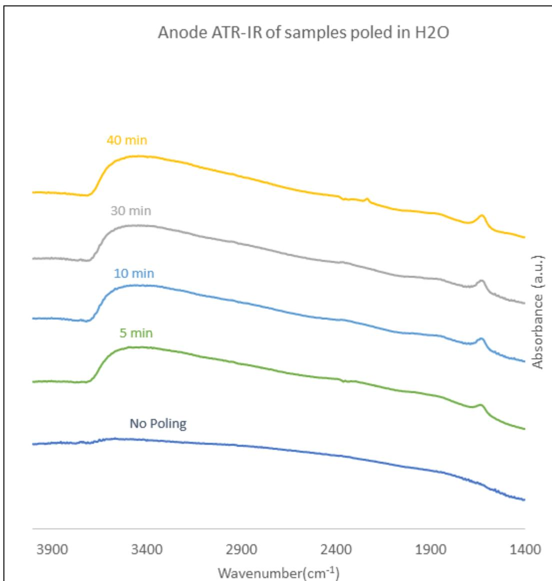
Figure 16: ATR-IR of anode side of glass samples poled for 0, 5, 10, 30 & 40 minutes. Data Credit: Jiawei Luo
