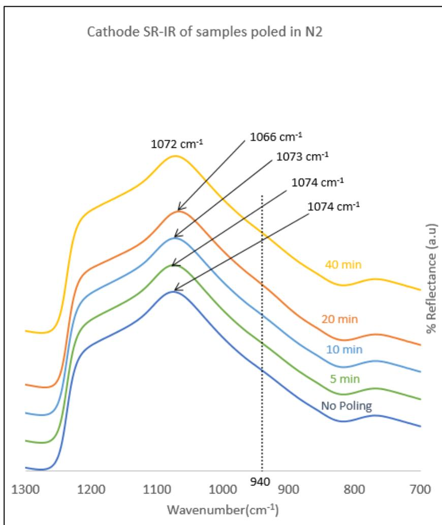
Figure 14: SR-IR spectra of samples poled in nitrogen environment for different poling times. Data Credit: Jiawei Luo.
