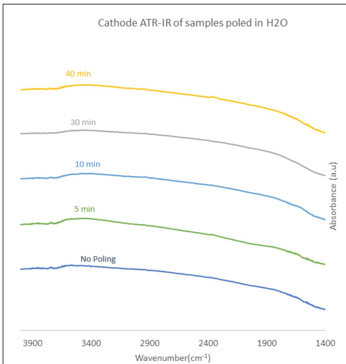
Figure 17: ATR-IR of cathode side of glass samples poled for 0, 5, 10, 30 & 40 minutes. Data Credit: Jiawei Luo
