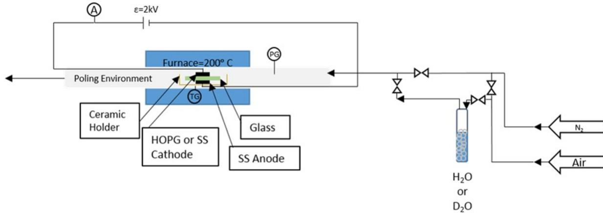
Figure 6: Thermal Poling apparatus diagram.
