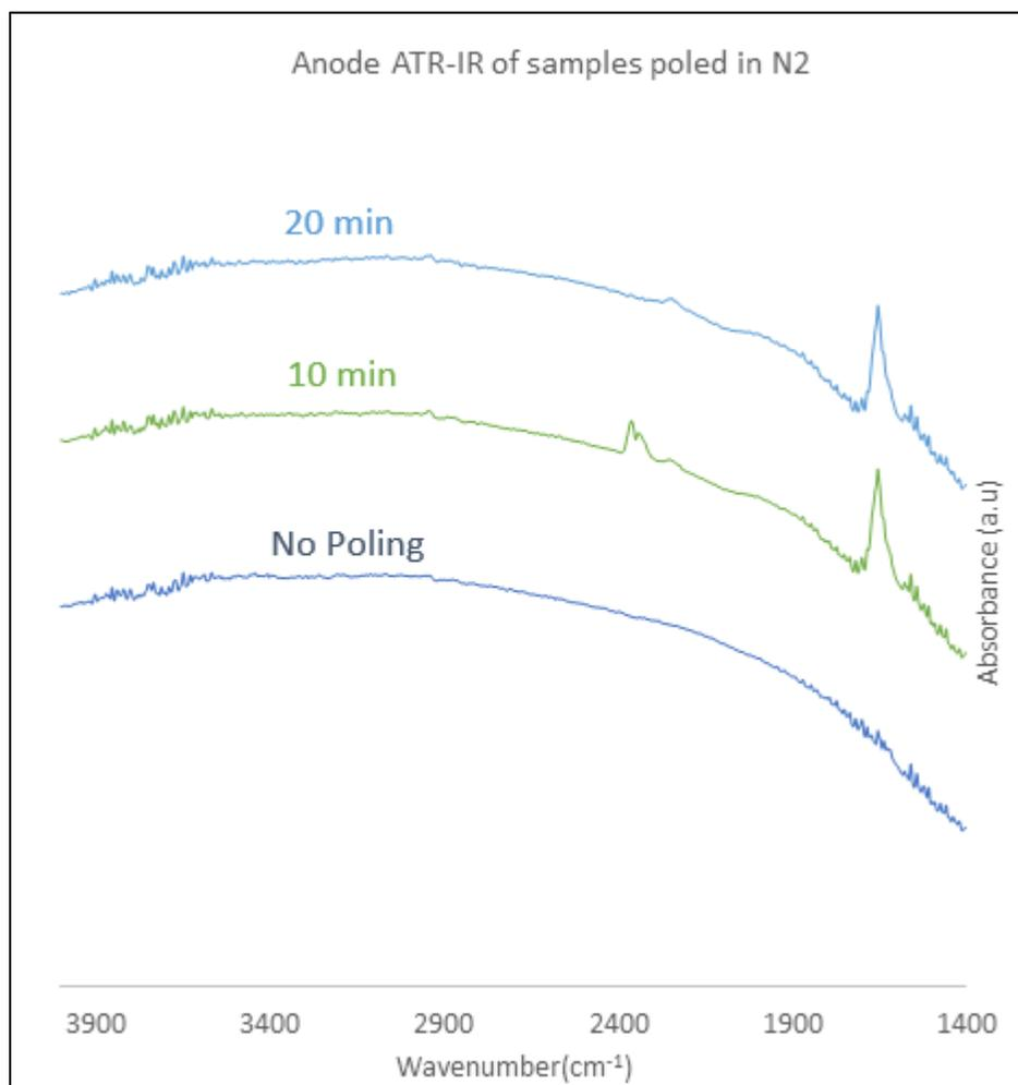
**Figure 19:** ATR-IR spectra of samples poled in nitrogen environment for 0, 10, and 20 minutes on anode side. Data Credit: Jiawei Luo.
