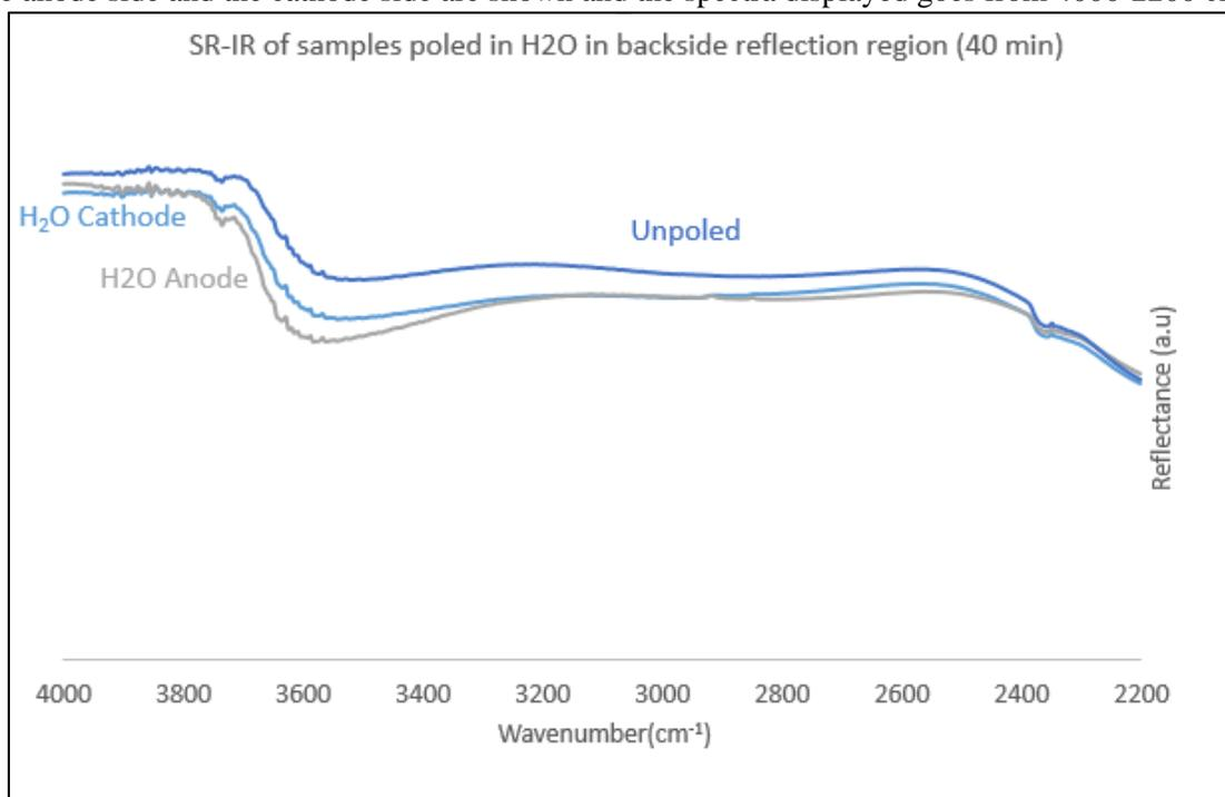
Figure 15: SR-IR spectra of sample poled in H<sub>2</sub>O environment taken on anode, cathode, and unpoled area of glass.
