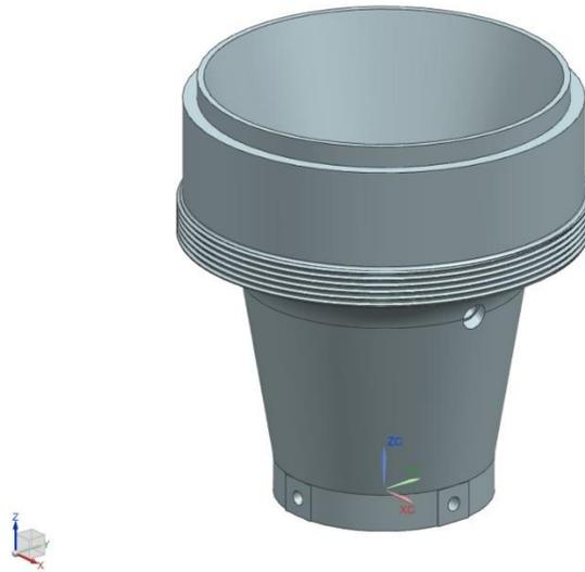
Figure 8: 3D CAD Nozzle Representation
